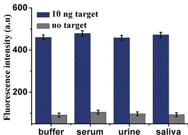
Fig. 6 Fluorescence intensity of the sensor for the detection of VEGF<sub>165</sub> in buffer and blank biological samples (human serum, urine and saliva, respectively). Error bars: SD,  $n = 3$ .
