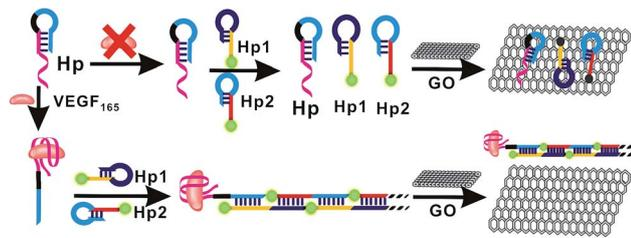
Fig. 1 Schematic illustration of the fluorescence assay detection of VEGF<sub>165</sub> based on target-triggered hybridization chain reaction amplification.
