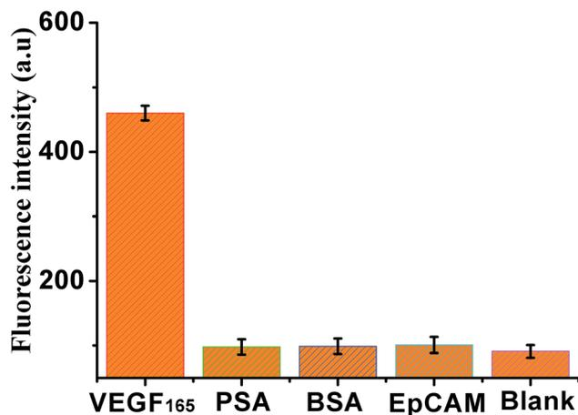
Fig. 5 Fluorescence intensity (at an emission wavelength of 519 nm) of the sensor in the presence of VEGF<sub>165</sub> (10 ng mL<sup>-1</sup>), PSA (100 ng mL<sup>-1</sup>), BSA (100 ng mL<sup>-1</sup>), EpCAM (100 ng mL<sup>-1</sup>) and black, respectively. Error bars: SD,  $n = 3$ .
