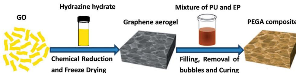
Fig. 1 The schematic fabrication process of PEGA composite.
