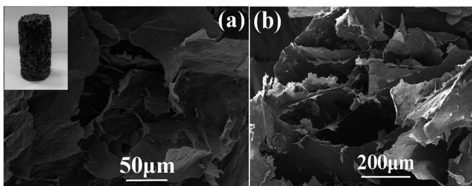
Fig. 4 Photo (inset picture in (a)) and SEM images ((a) and (b)) of the prepared graphene aerogel.
