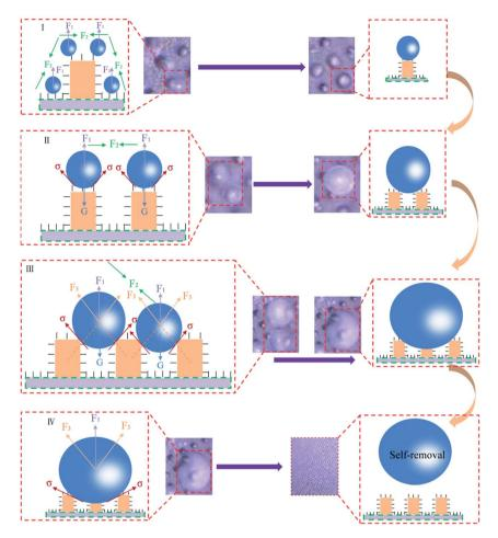
Fig. 8 The antifogging behaviors of the PF coupled with sprayed  $SiO_2$  coating and the MPA. Here,  $F_1$  is the repulsion force of the material itself,  $F_2$  is the intermolecular attraction,  $F_3$  is the repulsion force of the micro-pillared arrays,  $\sigma$  is surface tension and G is gravity.
