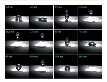
Fig. 4 Bounce dynamics of a water droplet impacting with the PF coupled with sprayed  ${\rm SiO_2}$  coatings and the MPA surface.
