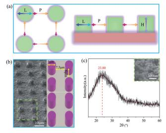
Fig. 2 (a) The top view (left) and side view (right) of the MPA. This pattern was repeated periodically across the PDMS surface. (b) The FESEM image of the fabricated  $SiO_2$ -sprayed MPA under low-magnification, demonstrating that the coated PDMS has a negligible effect on the global structure of the MPA. (c) The X-ray diffraction (XRD) spectrum of the coating and high-magnification FESEM image shows the nanoscale  $SiO_2$  (insert).
