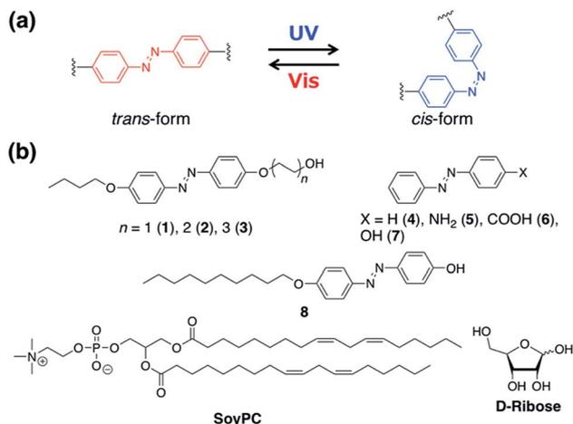
**Scheme 1** (a) Structural changes of the azobenzene moiety induced by UV and visible light irradiations. (b) Molecular structures of synthesized azobenzene derivatives (1–3, 8), azobenzene with and without polar substituents (4–7), SoyPC, and D-ribose.
