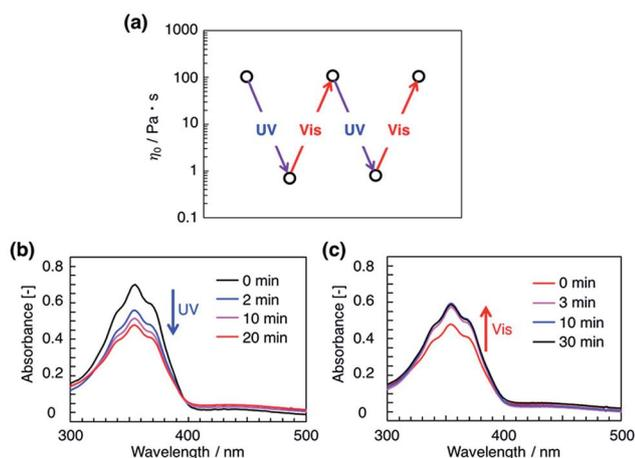
Fig. 2 Repeatability of zero-shear viscosity changes of a 15 mM 2/55 mM D-ribose/105 mM SoyPC/decane mixture upon UV and subsequent visible light irradiation (a). UV/vis absorption spectra of solutions after (b) UV and (c) subsequent visible light irradiation (the 2/ D-ribose/SoyPC/decane mixtures were diluted 400-fold with decane before the measurements).
