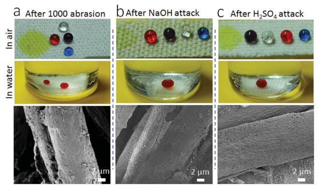
Fig. 5 Photos and SEM images of the coated fabric after, (a) 1000 cycles of abrasion, (b) immersing in NaOH solution (pH = 14) for 5 hours followed by rinsing with water and drying at 130 °C for 30 minutes, and (c) immersing in  $H_2SO_4$  solution (pH = 1) for 5 hours followed by rinsing with water and drying at 130 °C for 30 minutes (liquid droplets: yellow water, clear paraffin oil, red olive oil, purple mineral oil, and blue hexadecane).
