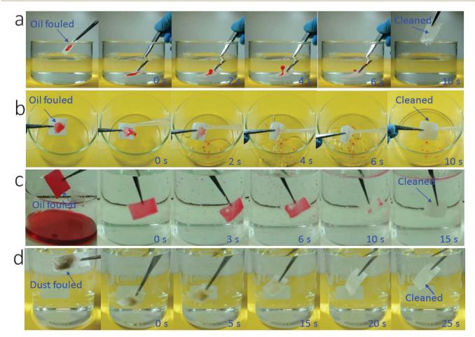
Fig. 4 Snapshots taken from videos to show cleaning of oil-contaminated fabrics with tap water, (a) pre-contaminated with a small amount of olive oil (50  $\mu$ L, the fabric was just immersed in water without shaking), (b) pre-contaminated with a small amount of olive oil (50  $\mu$ L, the fabric was rinsed with water), (c) olive oil fully fouled fabric after immersing and shaking in water, (d) dust-contaminated cotton fabric in water.
