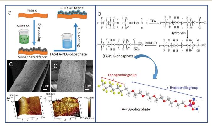
Fig. 1 (a) Schematic illustration of the procedure for coating treatment, (b) chemical reactions to synthesize FA-PEG-phosphate and the chemical structure of the synthesised FA-PEG-phosphate. (c and d) SEM images of: (c) uncoated cotton, (d) silica NP/FAS/FA-PEG-phosphate coated cotton. (e and f) AFM images of: (e) uncoated cotton, and (f) silica NP/FAS/FA-PEG-phosphate coated cotton.
