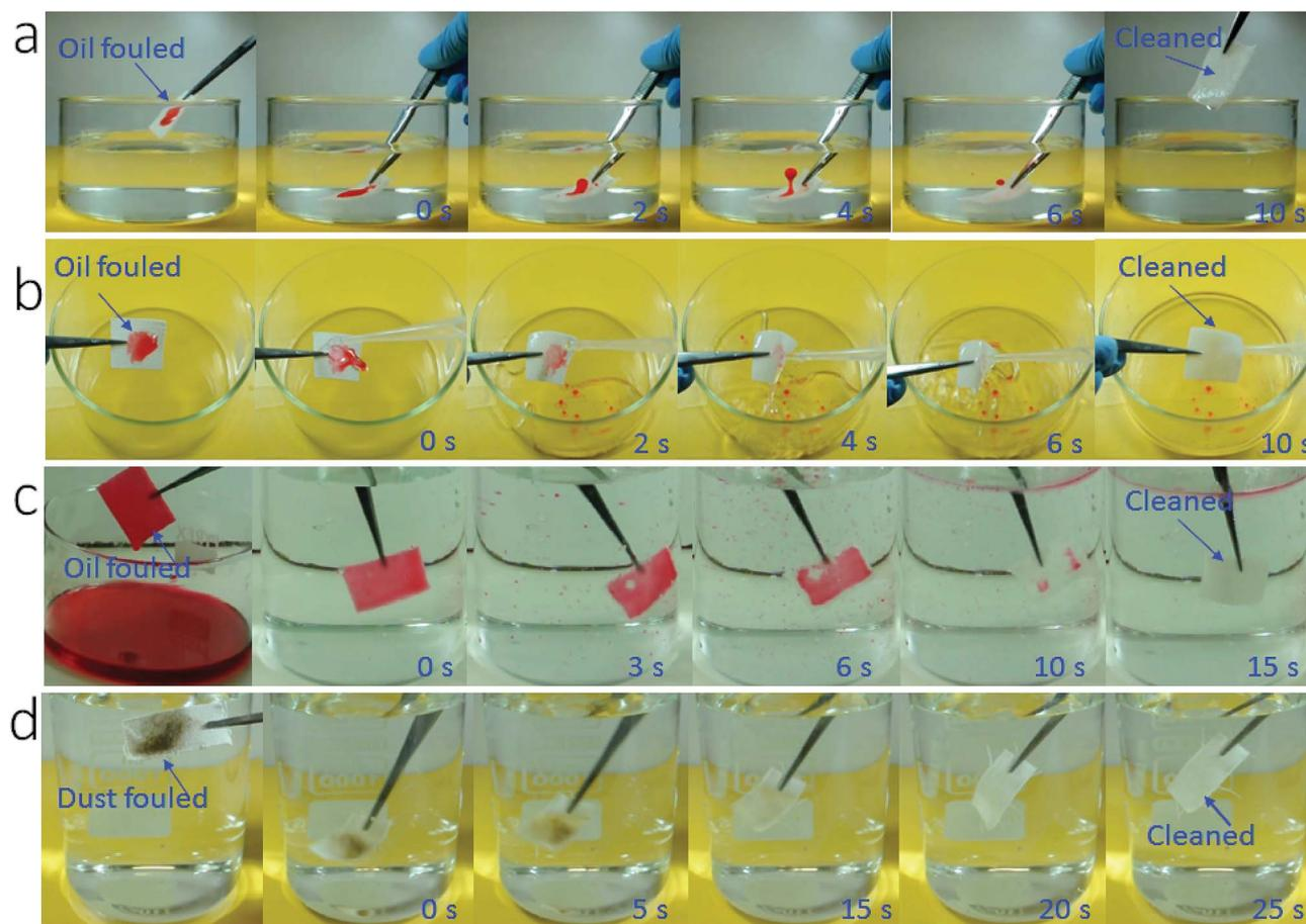
Fig. 4 Snapshots taken from videos to show cleaning of oil-contaminated fabrics with tap water, (a) pre-contaminated with a small amount of olive oil ( $50 \mu\text{L}$ , the fabric was just immersed in water without shaking), (b) pre-contaminated with a small amount of olive oil ( $50 \mu\text{L}$ , the fabric was rinsed with water), (c) olive oil fully fouled fabric after immersing and shaking in water, (d) dust-contaminated cotton fabric in water.
