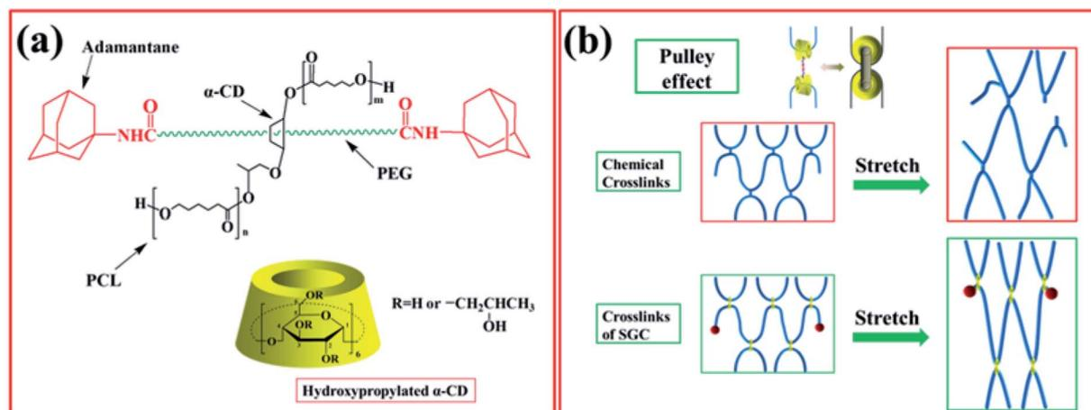
Fig. 2 (a) Chemical structure of SGC. (b) Schematic of the pulley effect.
