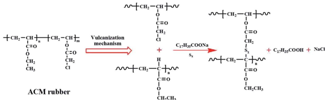
Fig. 3 Chemical structure and vulcanization mechanism of acrylic rubber.
