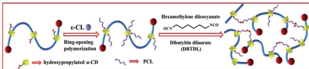
Fig. 1 Schematic of the preparation of SGC.
