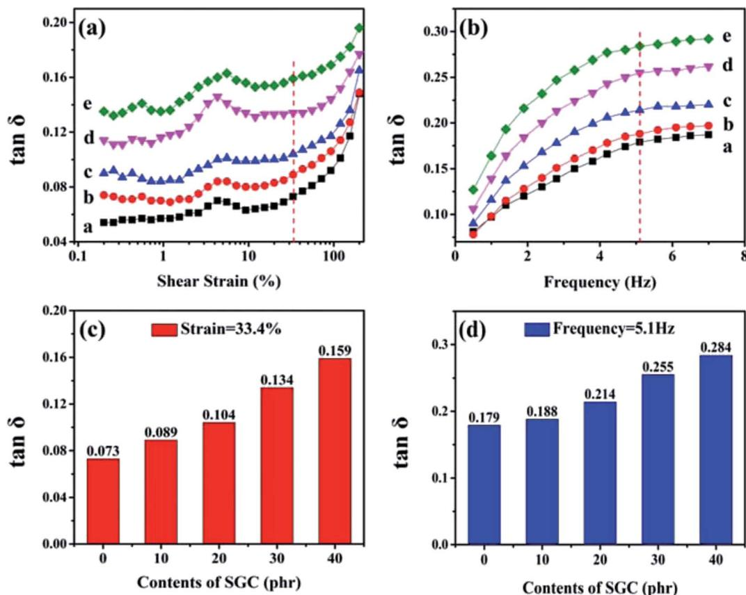
Fig. 9 RPA results of ACM/SGC composites: (a) variation of  $\tan \delta$  under dynamic shear strain sweep; (b) variation of  $\tan \delta$  under dynamic frequency sweep; (c)  $\tan \delta$  value of rubber composites at the same shear strain (33.4%); (d)  $\tan \delta$  value of rubber composites at the same frequency (5.1 Hz). (a) ACM; (b) ACM/SGC (100/10); (c) ACM/SGC (100/20); (d) ACM/SGC (100/30); (e) ACM/SGC (100/40).
