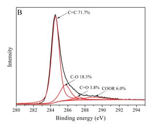
Fig. 1 (A) Raman spectra of SBA-15 and SBA-15-C; (B) C1s core level spectrum of SBA-15-C.
