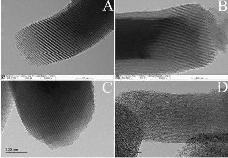
TEM images of SBA-15 (A), SBA-15-HC (B), SBA-15-C (C), and SBA-15-C etched by NaOH solution (D), and the scale bars were 100 nm.
