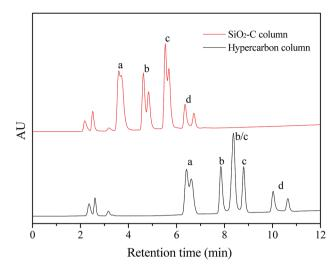
Fig. 7 The separation of oligosaccharide isomers on the  $SiO_2$ -C (5  $\mu$ m) and hypercarbon columns (150 mm  $\times$  4.6 mm): (a) LNnDFH-II, (b) LNDFH-I, (c) LNFP-II, (d) LNFP-I; (a and b) and (c and d) were two pairs of isomers, and each compound corresponded to double peaks due to the effect of  $\alpha/\beta$  anomeric splitting of saccharide.
