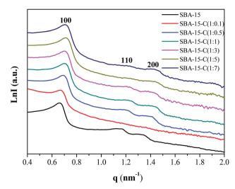
Fig. 5 SAXS patterns of SBA-15 and SBA-15-C under different substrate proportions.
