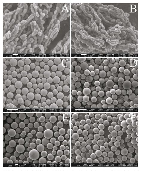
Fig. 2 SEM images of SBA-15 (A), SBA-15-C (B),  $SiO_2$  (5  $\mu$ m, C),  $SiO_2$ -C (5  $\mu$ m, D),  $SiO_2$  (30  $\mu$ m, E), and  $SiO_2$ -C (30  $\mu$ m, F), and the scale bars of (A and B) and (C-F) were 1 and 10  $\mu$ m, respectively.
