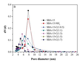
Fig. 4 Nitrogen adsorption/desorption isotherms and pore size distributions of SBA-15, SBA-15-NH $_2$  and SBA-15-C under different substrate proportions.
