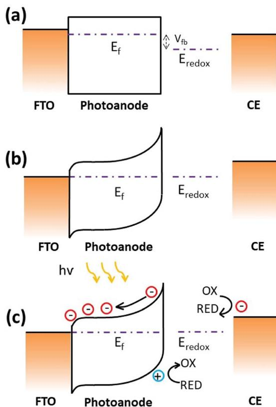
Fig. 5 Schematic energy band diagrams for flat band potential (a), and for SnSe<sub>2</sub> photoanode in contact with the SO<sub>4</sub><sup>2-</sup>/SO<sub>3</sub><sup>2-</sup> redox couple in the dark (b) and under illumination (c).  $E_f$  is the Fermi level energy.  $E_{redox}$  is the redox potential in the electrolyte (0.5 M Na<sub>2</sub>SO<sub>4</sub>). The counter electrode is Pt mesh.
