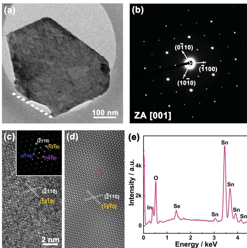
Fig. 2 (a) TEM image of a  $\text{SnSe}_2$  nanoflake. (b) SAED pattern of the  $\text{SnSe}_2$  nanoflake. (c) High-resolution TEM image of the  $\text{SnSe}_2$  nanoflake. Inset is the corresponding fast Fourier transform (FFT) from the TEM image along [001] zone axis. (d) Inverse FFT image of the  $\text{SnSe}_2$  nanoflake. (e) EDX spectrum of a  $\text{SnSe}_2$  nanoflake grown on FTO glass.
