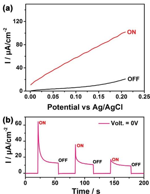
Fig. 3 (a) Linear sweep voltammograms of SnSe<sub>2</sub>/FTO electrode in dark and under illumination at the applied voltage between 0 V and 0.2 V versus Ag/AgCl electrode. (b) A typical current–time curve at 0 V versus Ag/AgCl electrode.
