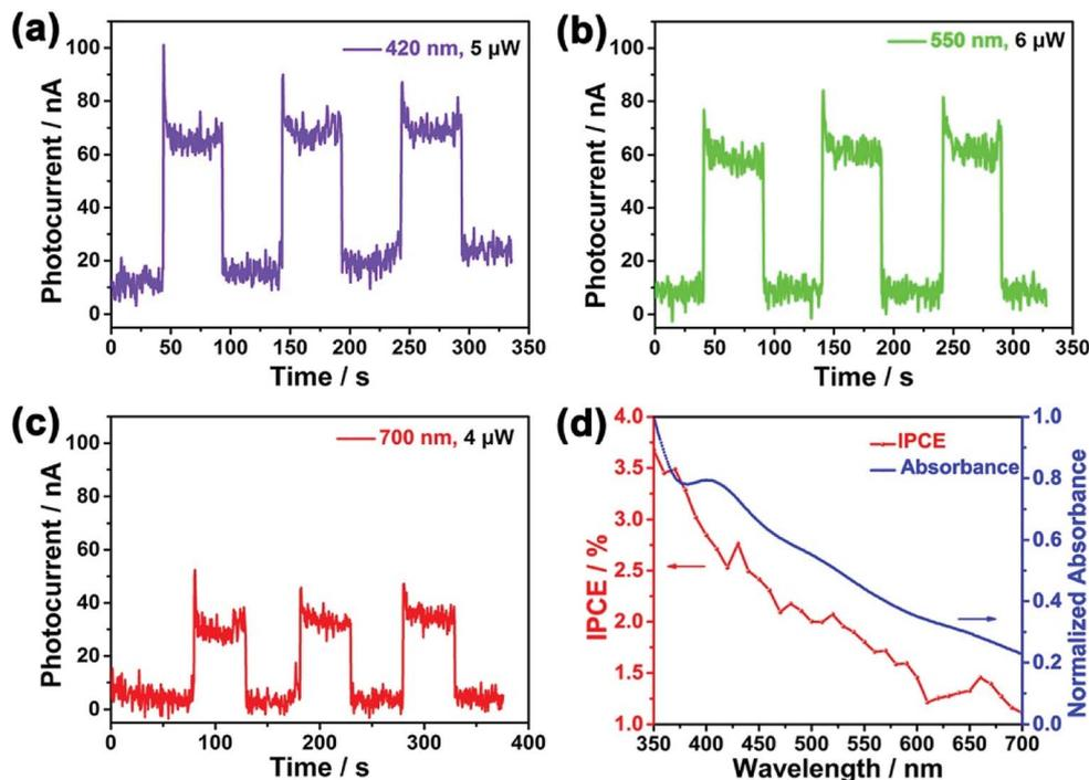
Fig. 4 Time-dependent photoresponse of SnSe<sub>2</sub> PEC under the illumination of selected wavelengths at the potential of 0 V vs. Ag/AgCl: (a) 700 nm, 4 μW; (b) 550 nm, 6 μW; (c) 420 nm, 5 μW. (d) Plot of IPCE spectrum (red line) and absorbance spectrum (blue line) versus wavelength at the potential of 0 V vs. Ag/AgCl electrode.
