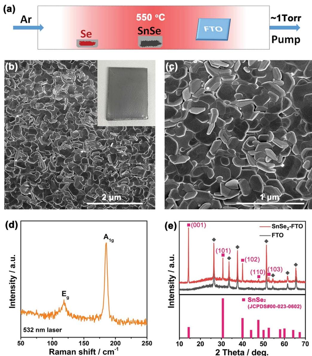
**Fig. 1** (a) Schematic illustration of the growth set up. (b and c) SEM images of as-grown SnSe<sub>2</sub> nanoflakes on FTO glass. Inset of (b) is an optical image of SnSe<sub>2</sub>/FTO glass. (d) Raman spectrum of as-grown SnSe<sub>2</sub> nanoflakes with 532 nm excitation laser. (e) XRD patterns for SnSe<sub>2</sub>/FTO glass and bare FTO glass. Bottom trace represents the powder diffraction patterns for SnSe<sub>2</sub> standard.
