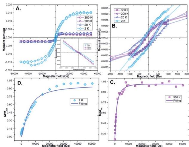
Fig. 2 Magnetic data. (A) Isothermal  $M - H$  loops obtained at different temperatures between 300 and 2 K. Inset shows magnetic hysteresis data without diamagnetic correction. (B) Closer view of the low magnetic field regions of the  $M - H$  loops. (C and D) Langevin fitting of 300 K and 2 K  $M - H$  curves respectively.
