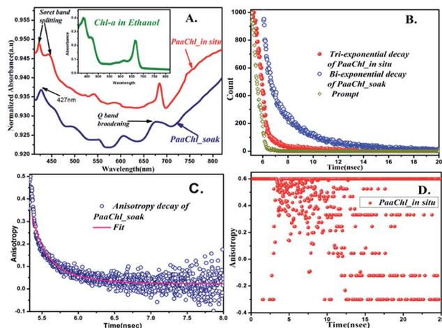
Fig. 1 Optical spectroscopy data of PaaChl (swollen and *in situ*; reprinted with permission). (A) UV-visible absorption spectra. (B) TCSPC data. (C) Fluorescence anisotropy decay of PaaChl<sub>soak</sub>. (D) Fluorescence anisotropy decay of PaaChl<sub>in situ</sub>.
