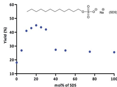
Fig. 2 Effect of SDS on the isolated yield of **6a** from the model laccase/TEMPO oxidation-U4CR system. Reaction conditions: benzyl alcohol (**1a**, 0.5 mmol), TEMPO (0.1 mmol), laccase from *Trametes versicolor* (15 mg), SDS (0.1 mmol) in 5 mL PBS (5.2 pH, 100 mM) were mixed for 24 h at room temperature. Then, *p*-methoxybenzylamine (**3a**, 0.5 mmol), phenylacetic acid (**4a**, 0.5 mmol) and *p*-methoxybenzyl isocyanide (**5a**, 0.5 mmol) were added and stirred for an additional 48 h.
