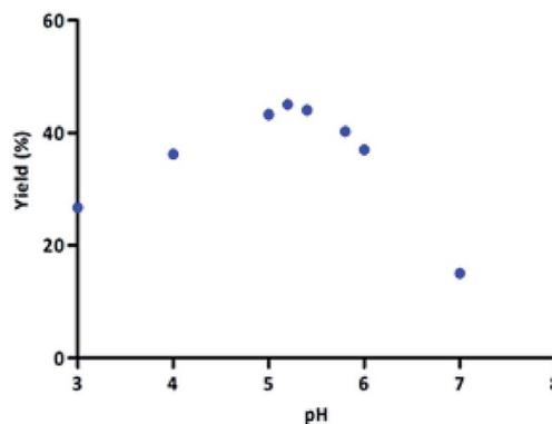
Fig. 1 Effect of pH on the isolated reaction yield of **6a** of the model laccase/TEMPO oxidation-U4CR system. Reaction conditions: benzyl alcohol (**1a**, 0.5 mmol), TEMPO (0.1 mmol), laccase from *Trametes versicolor* (15 mg), SDS (0.1 mmol) in 5 mL PBS (5.2 pH, 100 mM) were mixed for 24 h at room temperature. Then, *p*-methoxybenzylamine (**3a**, 0.5 mmol), phenylacetic acid (**4a**, 0.5 mmol) and *p*-methoxybenzyl isocyanide (**5a**, 0.5 mmol) were added and stirred for an additional 48 h.
