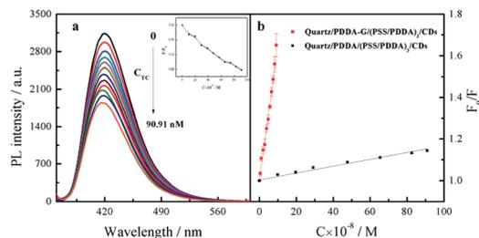
Fig. 9 (a) Fluorescence spectral response of quartz/PDDA-G/(PSS/PDDA)<sub>3</sub>/CDs SAMs toward Tc at different concentrations in 10 mM PB buffer of pH 6.8. (Inset graph shows the ratio  $F_0/F$  of fluorescence intensity varied with concentration of Tc). (b) Relationship curves between  $F_0/F$  of SAMs and Tc concentration.
