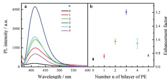
Fig. 6 (a) Fluorescence spectra of quartz/PDDA-G/(PSS/PDDA)<sub>*n*</sub>/CDs SAMs with different layers of (PSS/PDDA)<sub>*n*</sub> (*n* = 0–5). (b) Enhancement factor as a function of the number *n* of PSS/PDDA bilayers.
