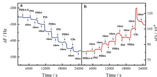
Fig. 3 Response in frequency (a) and dissipation (b) for fabrication process of quartz/PDDA-G/(PSS/PDDA)<sub>3</sub>/CDs SAMs.
