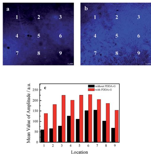
Fig. 5 Fluorescence microscopy images of (a) quartz/PDDA/(PSS/PDDA)<sub>3</sub>/CDs SAMs and (b) quartz/PDDA-G/(PSS/PDDA)<sub>3</sub>/CDs SAMs. (c) Confocal fluorescence values of quartz/PDDA/(PSS/PDDA)<sub>3</sub>/CDs SAMs and quartz/PDDA-G/(PSS/PDDA)<sub>3</sub>/CDs SAMs with different matching locations.
