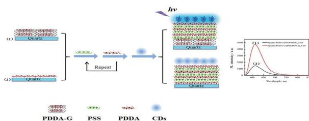
**Scheme 1** Schematic representation of assembly of (1) quartz/PDDA-G/(PSS/PDDA)<sub>3</sub>/CDs and (2) quartz/PDDA/(PSS/PDDA)<sub>3</sub>/CDs SAMs.
