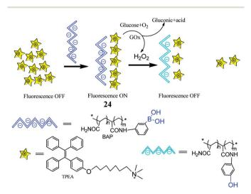
Fig. 3 Cartoon illustrating sensor 24 detecting glucose.<sup>72</sup>
