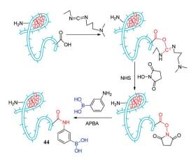
Fig. 7 Formation of boronic acid conjugated gold nanoclusters (sensor 44).<sup>103</sup>
