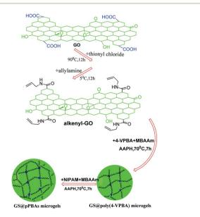
Fig. 14 Schematic illustration for the synthesis of GS@poly(4-VPBA) and GS@pPBAs microgels.151
