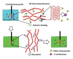
Fig. 16 Schematic illustration of saccharides sensing by means of the PBA-functionalized CNTs.<sup>161</sup>
