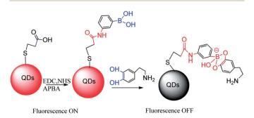
Fig. 13 Boronic acid QDs synthesis and dopamine detection diagram.150
