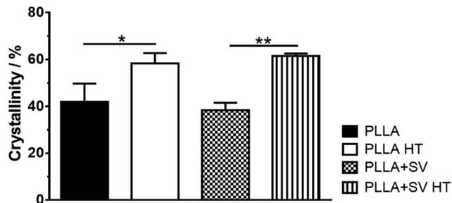
Fig. 4 Crystallinity of electrospun membranes. \* =  $p < 0.05$ ; \*\* =  $p < 0.01$ .
