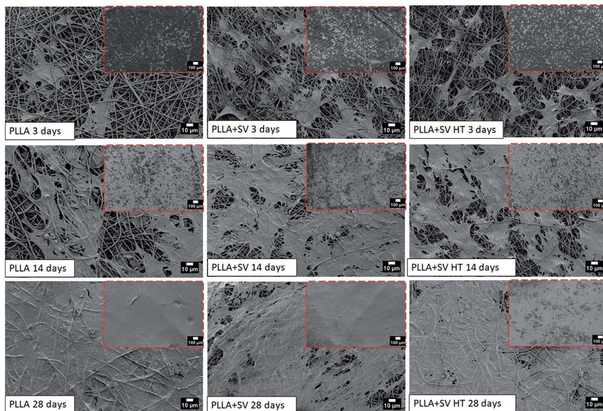
Fig. 6 SEM images of rBMSCs cultured on the membranes at 150 $\times$  (red squares) and 1000 $\times$ .
