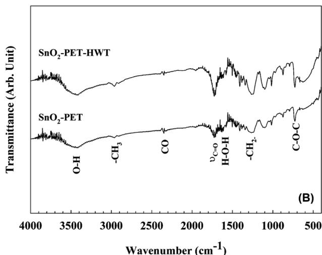
Fig. 4 The FT-IR spectra of SnO<sub>2</sub>. (A) SnO<sub>2</sub>-G before and after the HWT process, (B) SnO<sub>2</sub>-PET before and after the HWT process.
