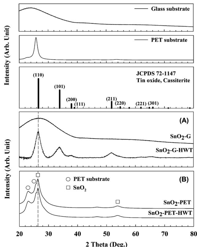
Fig. 8 The XRD patterns of SnO<sub>2</sub> (JCPDS 72-1147), the glass and PET substrate. (A) XRD patterns of the glass substrate and SnO<sub>2</sub>-G before and after the HWT process, (B) XRD patterns of the SnO<sub>2</sub>-PET before and after the HWT process.
