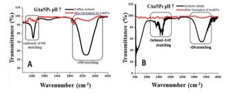
Fig. 5 FTIR spectra of (A) GAuNPs and (B) CAuNPs fabricated at pH 7 of the reaction mixtures. The spectra corresponding to pH adjusted reaction mixture before the formation of NPs are also presented as reference (black)
