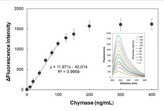
Fig. 5 Detection of chymase activity assay by AuNPs-peptide probe. AuNPs-peptide probe was incubated with various concentrations of chymase (0–400 ng mL $^{-1}$ ) for 15 min at 37 °C, pH 8.0. The linear correlation between 10 and 100 ng mL $^{-1}$  chymase was within confidence limits. Error bars (SD) represent data from three independent detections. The inserted figure shows fluorescence emission spectra of AuNPs-peptide probes activated by different concentrations of chymase.
