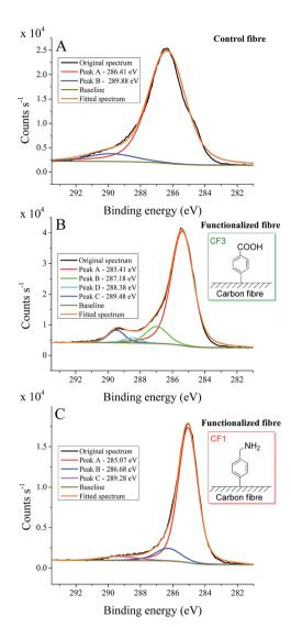
Fig. 1 High-resolution C1s spectra with curve fitting for control sample (A), functionalized carbon fibre CF3 (B) and CF1 (C).
