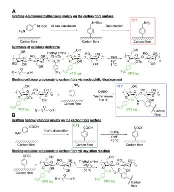
Scheme 1 Synthetic strategies to covalently bind cellulose propionate to the carbon fibre surface. Nucleophilic displacement (A) and acylation approach (B).
