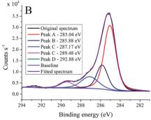
Fig. 2 High-resolution F1s (A) and C1s (B) spectra of cellulose propionate-functionalized carbon fibre samples (CF2).
