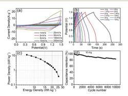
Fig. 7 (a) CV curves of  $Co_9S_8/CNF-3//ACNFs$  capacitor at various scan rates; (b) galvanostatic charge—discharge curves of  $Co_9S_8/CNF-3//ACNFs$  capacitor at different current densities; (c) Ragone plots of  $Co_9S_8/CNF-3//ACNFs$  capacitor; and (d) cycling retention curves of  $Co_9S_8/CNF-3//ACNFs$  capacitor at a current density of 10 A g-1 for 10 000 cycles.
