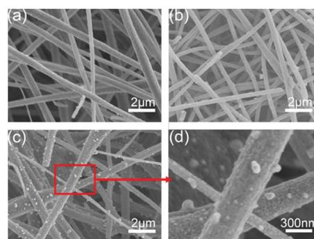
Fig. 3 SEM images of the  $\text{Co}_9\text{S}_8/\text{CNF}$  samples, (a)  $\text{Co}_9\text{S}_8/\text{CNF}$ -1, (b)  $\text{Co}_9\text{S}_8/\text{CNF}$ -2, (c) and (d)  $\text{Co}_9\text{S}_8/\text{CNF}$ -3.
