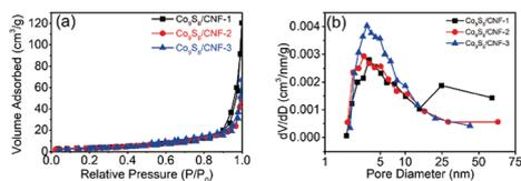
Fig. 5 (a)  $\text{N}_2$  adsorption/desorption isothermal curves for  $\text{Co}_9\text{S}_8/\text{CNF}$  samples, and (b) the corresponding pore size distributions calculated from the adsorption branch.
