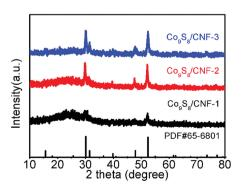
Fig. 1 XRD pattern of the Co<sub>9</sub>S<sub>8</sub>/CNF samples.
