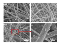
Fig. 3 SEM images of the Co<sub>9</sub>S<sub>8</sub>/CNF samples, (a) Co<sub>9</sub>S<sub>8</sub>/CNF-1, (b)  $Co_9S_8/CNF-2$ , (c) and (d)  $Co_9S_8/CNF-3$ .
