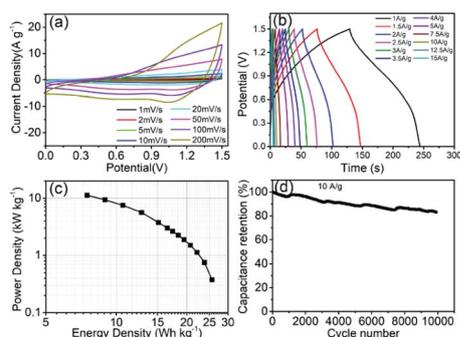
Fig. 7 (a) CV curves of  $\text{Co}_9\text{S}_8/\text{CNF-3}/\text{ACNFs}$  capacitor at various scan rates; (b) galvanostatic charge–discharge curves of  $\text{Co}_9\text{S}_8/\text{CNF-3}/\text{ACNFs}$  capacitor at different current densities; (c) Ragone plots of  $\text{Co}_9\text{S}_8/\text{CNF-3}/\text{ACNFs}$  capacitor; and (d) cycling retention curves of  $\text{Co}_9\text{S}_8/\text{CNF-3}/\text{ACNFs}$  capacitor at a current density of  $10 \text{ A g}^{-1}$  for 10 000 cycles.
