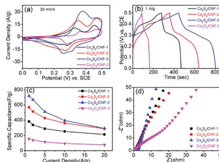
Fig. 6 (a) CV curves of the  $\text{Co}_9\text{S}_8/\text{CNF}$  and  $\text{Co}_3\text{O}_4/\text{CNF}$  electrodes at  $20 \text{ mV s}^{-1}$  scan rate, (b) GCD curves of the  $\text{Co}_9\text{S}_8/\text{CNF}$  and  $\text{Co}_3\text{O}_4/\text{CNF}$  electrodes at  $1 \text{ A g}^{-1}$  current density, (c) the specific capacitance versus current densities and (d) the EIS spectra of different electrodes.
