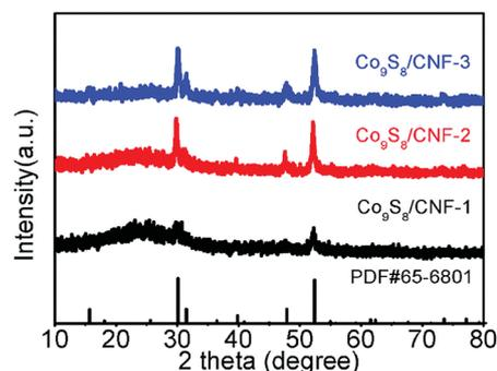
Fig. 1 XRD pattern of the Co<sub>9</sub>S<sub>8</sub>/CNF samples.
