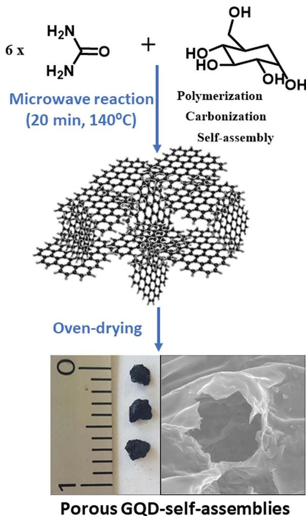
Scheme 1 Synthetic procedure of the GQD-assemblies *via* microwave-assisted one-pot reaction.
