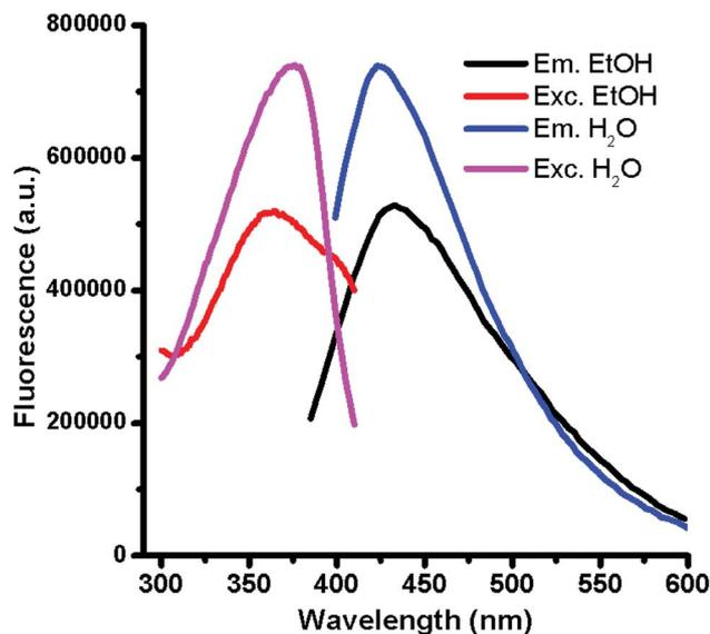
Fig. 1 Fluorescence spectra of GQDs after 20 minutes of microwave reaction. Excitation and emission curves of well-dispersed GQD in water and ethanol are shown ( $1 \text{ mg mL}^{-1}$ ,  $\lambda_{\text{ex}} = 375 \text{ nm}$ , Slits at 2 nm).
