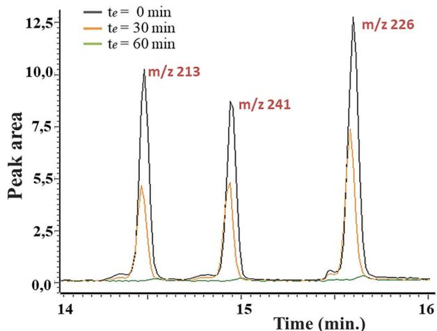
Fig. 6 Stacked chromatograms of different herbicides ( $m/z$  213 for simetryn,  $m/z$  241 for prometryn and  $m/z$  226 for terbutryn) upon concentration of  $1 \text{ mg L}^{-1}$  and at different contact.
