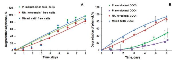
Fig. 6 (A) Degradation of phenol by the suspension of *P. mendocina, Rh. koreensis* and their mixture (1 : 1). (n = 2), (B) degradation of phenol by *P. mendocina* CCC3 and CCC4 with a crosslinked number of cells equal to  $5 \times 10^8$ , *Rh. koreensis* CCC4 and their mixture CCC3 (1 : 1) (n = 2).
