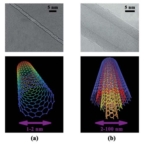
Fig. 1 Transmission electron microscopy images and schematic diagrams of carbon nanotubes, showing typical diameters of (a) a single-walled carbon nanotube and (b) a multi-walled carbon nanotube. The microscopy image of the single-walled carbon nanotube is adapted with permission from ref. 5. Copyright 2012, Springer Nature Limited. The microscopy image of the multi-walled carbon nanotube is adapted from the "Endo Laboratory" website.6
