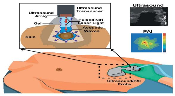
Fig. 7 Integrated real-time photoacoustic/ultrasound imaging
