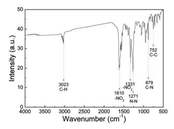
Fig. 6 IR spectra of samples.
