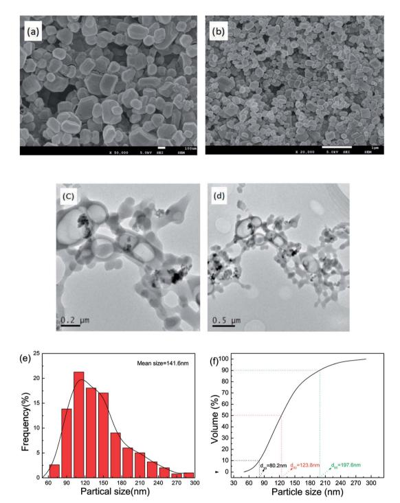
SEM and TEM images and particle size distribution of nano CL-20/RDX co/mixed crystals.
