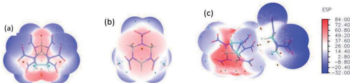
Fig. 2 Molecular electrostatic potential distribution of the structures of explosives: (a) CL-20, (b) RDX, (c) CL-20/RDX.
