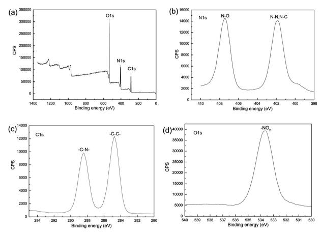
Fig. 7 XPS spectrum of the nano CL-20/RDX co/mixed crystal
