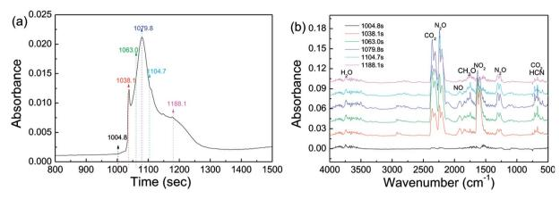
Fig. 9 DSC-IR spectra of CL-20/RDX: (a) the DSC curve in DSC-IR analysis; (b) IR spectra of gas products intercepted at different times.
