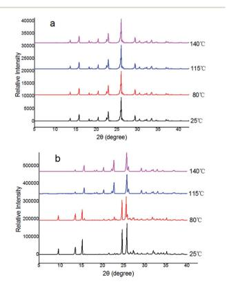
Fig. 4 In situ variable-temperature powder X-ray diffraction patterns for the polymorphs: (a) Form I, (b) conversion of Form II  $\rightarrow$  Form I.
