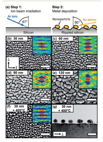
Fig. 1 Morphology of self-organized gold nanostructures on rippled templates. (a) Illustration of two-step fabrication routine. (b-f) Topview SEM images for different gold thicknesses from 30 nm to 120 nm and (f) 30 nm with post-annealing at 400 °C. The insets show the corresponding 2D autocorrelations. (g) Cross-sectional bright-field TEM image of (f). Scale bars (b-f): 200 nm (insets 50 nm), (g) 50 nm.
