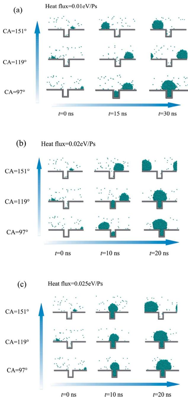
Fig. 7 Droplet nucleation and growth on the rough surface for three different contact angles (CA). (a) Heat flux =  $0.01 \text{ eV ps}^{-1}$ ; (b) heat flux =  $0.02 \text{ eV ps}^{-1}$ ; (c) heat flux =  $0.025 \text{ eV ps}^{-1}$ .
