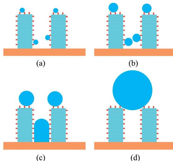
Fig. 10 The schematic of droplet nucleation and growth on the micro-nanostructured surface for  $r_c > S$ . (a) Droplet nucleation outside the nanostructures; (b) droplet growth due to the vapour condensation; (c) droplet growth due to coalescence; (d) the formation of Cassie droplet.
