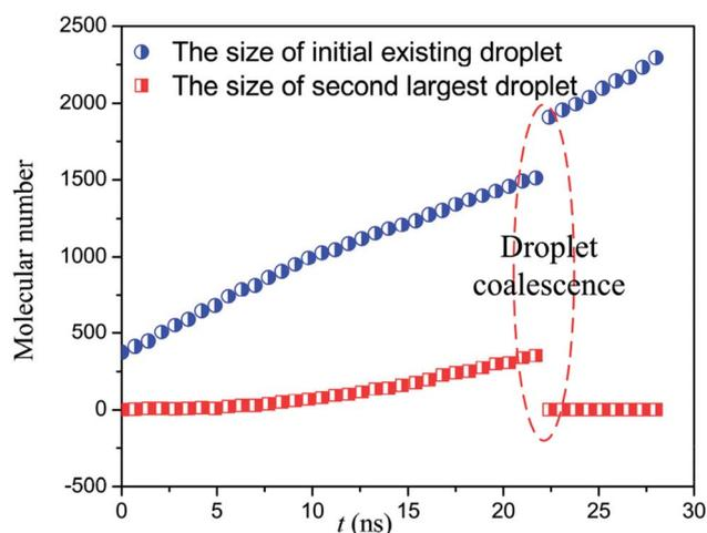
Fig. 6 The size of the initial droplet and the second largest droplet under heat flux of  $0.02 \text{ eV ps}^{-1}$ .
