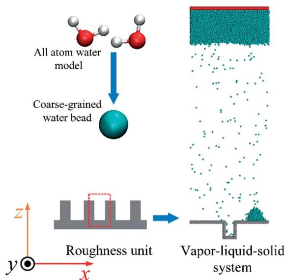
Fig. 1 The setup of the simulation system.
