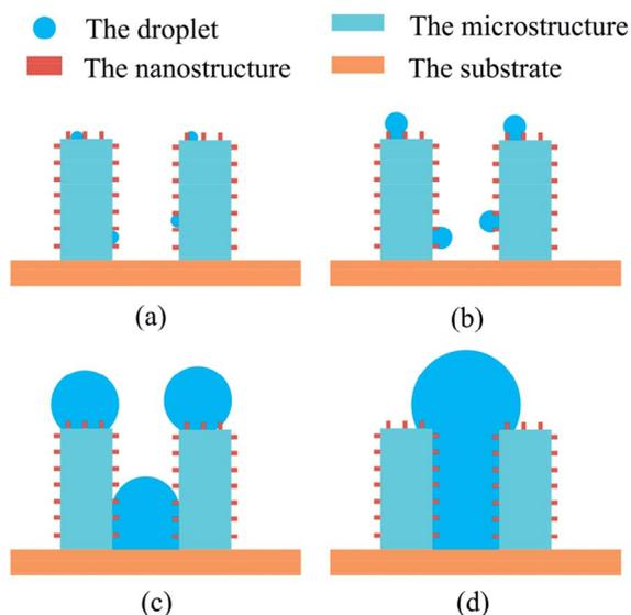
Fig. 9 The schematic of droplet nucleation and growth on the micro-nanostructured surface for  $r_c < S$ . (a) Droplet nucleation inside the nanostructures; (b) droplet growth due to the vapour condensation; (c) droplet growth due to coalescence; (d) the formation of Wenzel droplet.
