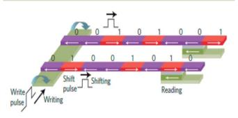
Fig. 13 Schematic of racetrack memory. A write pulse on the left produces magnetic fields to reverse the magnetization in the desired direction. A shift pulse exerts spin-transfer torque and shifts all the domain walls in the same direction. Reading is done with a magnetic tunnel junction. Figure reproduced with permission from Thomas et al., (2011).<sup>95</sup>
