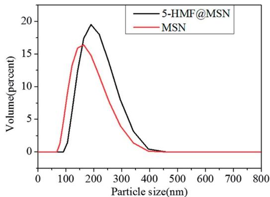
Fig. 6 Particle size distribution of MSN and 5-HMF@MSNs.
