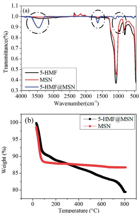
Fig. 7 (a) FT-IR spectra of pristine MSNs and 5-HMF@MSNs. (b) TGA curves of and MSNs, 5-HMF@MSNs.
