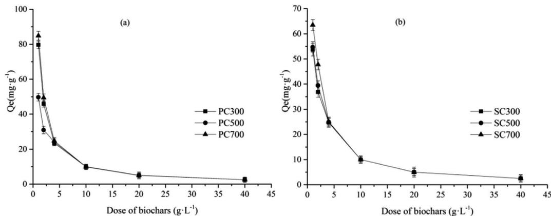
Fig. 4 Effects of biochar mass on the adsorption of Cd(II) by different spent *Pleurotus ostreatus* substrate biochars (a) and spent shiitake substrate biochars (b). Note: spent *Pleurotus ostreatus* substrate biochar (PC), spent shiitake substrate biochar (SC).
