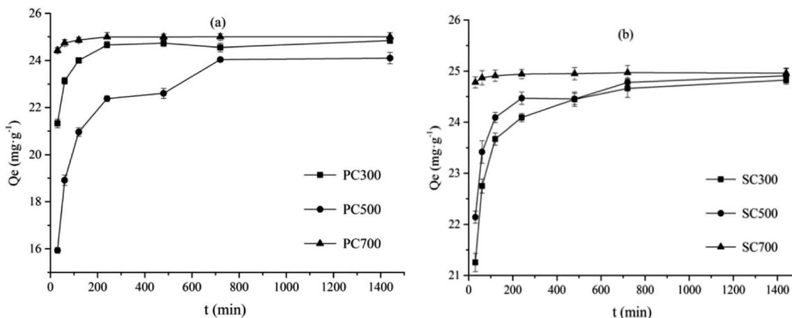
Fig. 2 Adsorption kinetics of Cd(II) onto the different spent *Pleurotus ostreatus* substrate biochar (a) and spent shiitake substrate biochar (b). Note: spent *Pleurotus ostreatus* substrate biochar (PC), spent shiitake substrate biochar (SC).
