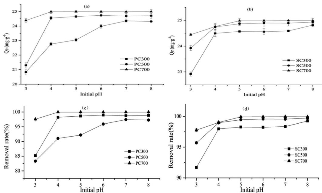
Fig. 5 Effects of initial pH on Cd(II) adsorption capacity by different spent *Pleurotus ostreatus* substrate biochars (a) and spent shiitake substrate biochars (b). And the effect of pH on removal rate of Cd(II) by different spent *Pleurotus ostreatus* substrate biochars (c) and spent shiitake substrate biochars (d). Note: spent *Pleurotus ostreatus* substrate biochar (PC), spent shiitake substrate biochar (SC).
