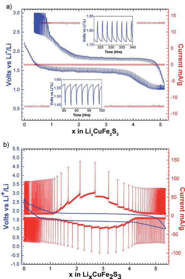
Fig. 3 (a) Potential–composition curve of  $\text{CuFe}_2\text{S}_3$  performed in a galvanostatic intermittent mode (GITT) with a rate of C/40 for 15 min and relaxation period of 2 h, (b) potentiometric titration curve (PITT) in the range of 3.0–1.0 V vs.  $\text{Li}^+/\text{Li}$  using 5 mV potential step in duration of 1 h and current limitation equivalent to a galvanic current  $I_{\text{limit}} = I_{\text{C}/100}$ .
