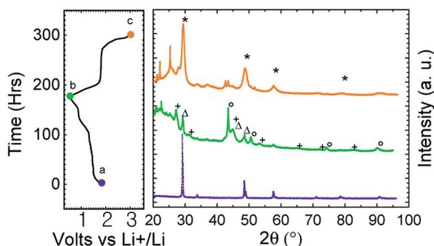
Fig. 4 Powder X-ray diffraction patterns of (a) as prepared isocubanite  $\text{CuFe}_2\text{S}_3$ , (b) discharged phase down to 0.5 V (C/20) (c) charged phase up to 3.0 V (C/20).  $\text{Cu}_x\text{Fe}_y\text{S}_z$  (\*),  $\text{Li}_2\text{S}$  (+), Cu (○), Fe (Δ) and undefined products (□).
