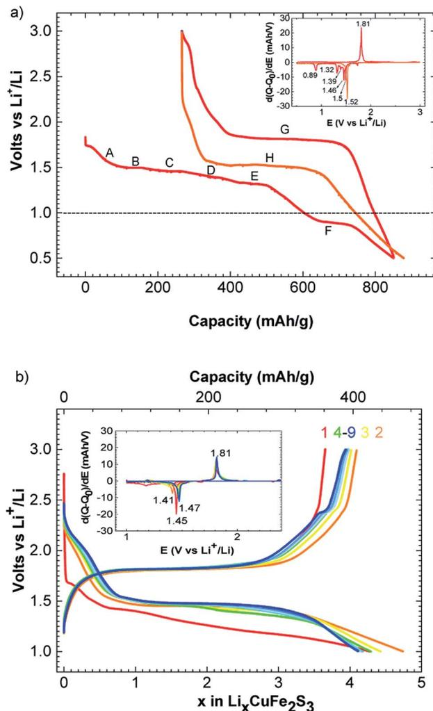
Fig. 2 Voltage–composition curve for  $\text{CuFe}_2\text{S}_3$  in the potential window 3.0–0.5 V at C/20/Li and inset: derivative curve  $|dQ/dE|$  vs. voltage (a); voltage–composition curve for  $\text{CuFe}_2\text{S}_3$  in the potential window 3.0–1.0 V at C/2/Li and its corresponding derivative curve  $|dQ/dE|$  vs. voltage (b).
