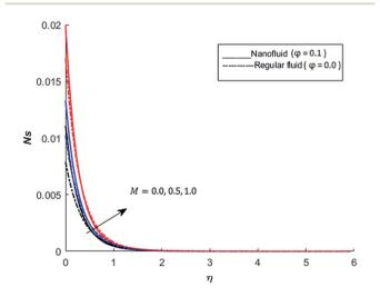
Fig. 30 The effect of M on the entropy generation when Pr=0.3, Bi=0.1, Nr=0.2, Gr=5, Gr=5
