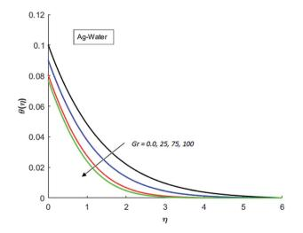
Fig. 20 Temperature curves for various value of Gr when M = 0.5, Pr =0.3. Ec = 0.5. Nr = 0.2 and  $\lambda = 1$ .
