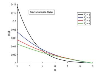
Fig. 26 Temperature curves for various value of Nr when M = 0.5, Pr = 0.3. Ec = 0.1. Gr = 0.5 and  $\lambda$  = 1.
