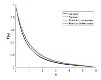
Fig. 13 Velocity profiles for different nanofluids when M=0.5, Pr=0.3, Ec = 0.1, Gr = 5, Nr = 0.2 and  $\lambda$  = 1.
