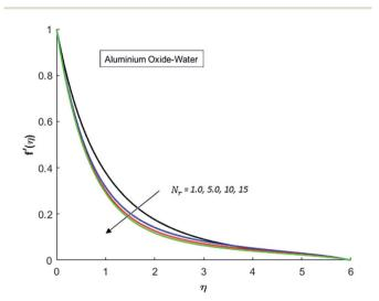
Fig. 11 Velocity distribution for various value of Nr when M = 0.5, Pr = 0.3. Gr = 0.5. Ec = 0.1 and  $\lambda$  = 1.
