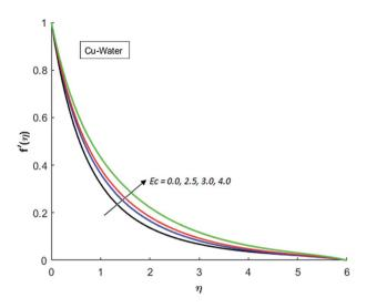
Fig. 1 Velocity distribution for various value of Ec when M=0.5, Pr = 0.3, Gr = 5, Nr = 0.2 and  $\lambda=1$ .
