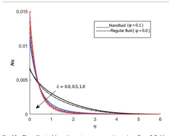
Fig. 29 The effect of  $\lambda$  on the entropy generation when Pr = 0.3, M = 1, Bi = 0.1, Nr = 0.2, Gr = 5, Ec = 0.5, Re = 1, Br = 1 and  $\Omega$  = 1.
