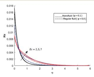
Fig. 27 The effect of Eckert number Ec on the entropy generation when Pr=0.3, M=1, Bi=0.1, Nr=0.2, Gr=5, A=1, Re=1, Br=1 and Q=1
