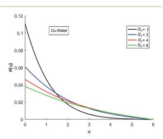
Fig. 23 Temperature curves for various value of Nr when M = 0.5, Pr = 0.3, Ec = 0.1, Gr = 0.5 and  $\lambda = 1$ .
