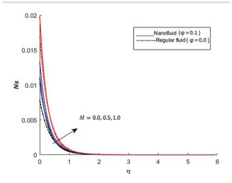
Fig. 30 The effect of M on the entropy generation when Pr=0.3, Bi=0.1, Nr=0.2, Gr=5, Cr=5, Cr=5
