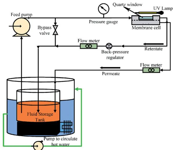
Fig. 1 A schematic of photocatalytic UF system (operational pressure: 0.1 MPa, cross-flow rate: 0.5 L min<sup>-1</sup>).
