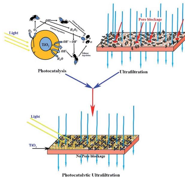
Fig. 10 Schematic of the photocatalytic UF process.
