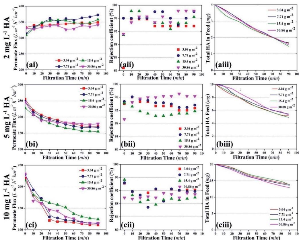
Fig. 5 Effect of various concentrations of HA on the photocatalytic UF process; the initial 'a', 'b', and 'c' represent 2 mg L<sup>-1</sup>, 5 mg L<sup>-1</sup>, and 10 mg L<sup>-1</sup> HA concentration, respectively; the numeric 'i', 'ii', and 'iii' represent permeate flux, rejection coefficient, and the decrease in HA quantity in the total feed volume, respectively.
