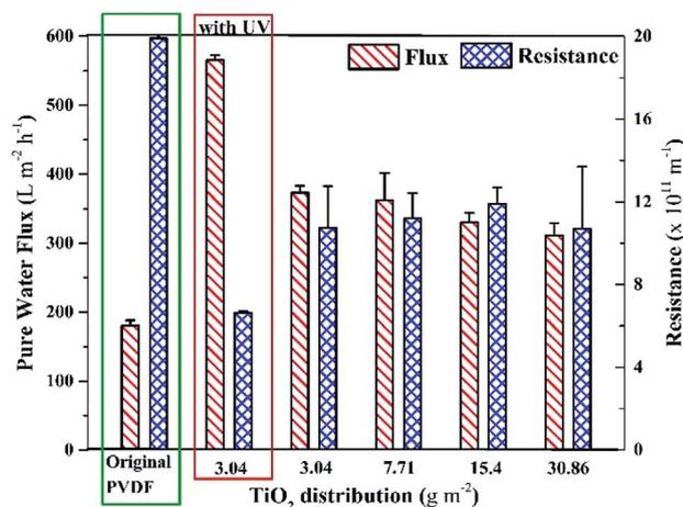
Fig. 3 Pure water flux and internal resistances of the membranes with different distribution amount of surface-located TiO<sub>2</sub> NPs in comparison with the original PVDF membrane.
