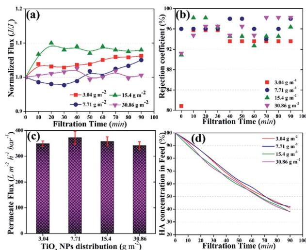
Fig. 4 Photocatalytic UF results of the membranes with different distribution amounts of TiO<sub>2</sub> NPs; (a) normalized fluxes of the membranes, (b) rejection coefficients of the membranes for HA, (c) permeate fluxes of the membranes at the end of the UF, (d) HA percentage in the feed tank as a factor of time, the total amount of HA in the feed was 4 mg.
