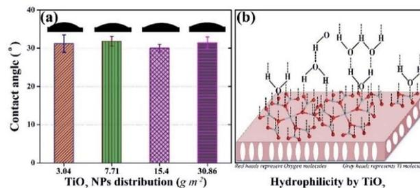
Fig. 2 Hydrophilic potential of membranes with surface located TiO<sub>2</sub> NPs: (a) contact angle values of membranes with different distributions of TiO<sub>2</sub> NPs; (b) schematic of the hydrophilic mechanism by TiO<sub>2</sub>.
