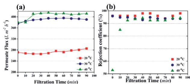
Fig. 7 The effect of temperature on photocatalytic UF (distribution amount of TiO<sub>2</sub> NPs was 3.04 g m<sup>-2</sup> and HA concentration in the feed was 2 mg L<sup>-1</sup>). (a) Permeate flux as a factor of filtration time. (b) Rejection coefficient for HA with different filtration time.
