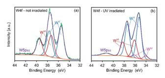
Fig. 4 XPS spectra of CTA-W<sub>12</sub> showing binding energies for W 4f energy levels in (a) un-irradiated and (b) UV-irradiated (3 h) material.
