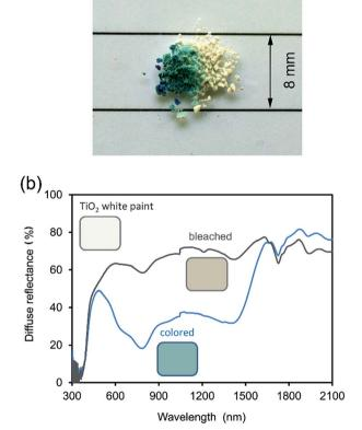
Fig. 2 Photochromic properties of CTA-W<sub>12</sub>. (a) Blue color developed when 315 nm UV source was directed onto the side of a sample of dry powder. (b) UV-vis diffuse reflectance spectra of CTA-W<sub>12</sub> as-prepared and after 1 hour of UV exposure. The diffuse reflectance scale has been calibrated with a white TiO<sub>2</sub> sample and converted to approximate RGB colors via the CIE L-a\*-b\* color scale.
