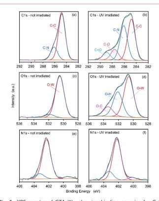
Fig. 5 XPS spectra of CTA- $W_{12}$  showing binding energies for C 1s energy levels in (a) un-irradiated and (b) UV-irradiated (3 h) material, O 1s energy levels in (c) un-irradiated and (d) UV irradiated, and N 1s energy levels in (e) un-irradiated and (f) UV-irradiated.
