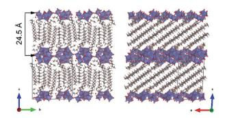
Fig. 1 A schematic depiction of the structure of CTA-W<sub>12</sub> showing planes of hexagonally-packed Keggin ions with intercalated and interdigitated cetyltrimethylammonium chains (see Colusso et al.21 for further discussion.).
