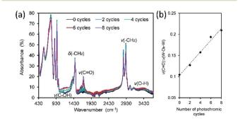
(a) FTIR spectra of CTA-W<sub>12</sub> and after 0, 2, 4, 6 and 8 photochromic cycles (1 cycle = 1 h UV exposure followed by 23 h in dark ambient). (b) Plot of  $\nu(C=O)$ :  $\nu(W-O_b-W)$  peak area ratio versus number of photochromic cycles
