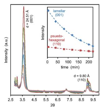
Fig. 6 In situ low-angle synchrotron P-XRD patterns of CTA-W<sub>12</sub> continually irradiated by UV light. The  $2\theta$  values are scaled for comparison with Cu Ka data. The lamellar (001) and pseudo-hexagonal (110) POM peaks appear at d = 24.51 Å and d = 9.80 Å, respectively. Inset. Interlamellar (001) and pseudo-hexagonal (110) peak height as a function of exposure time.
