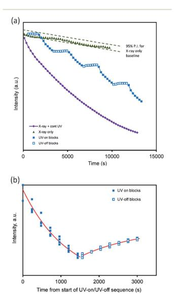
Fig. 7 Changes on application of UV-irradiation during continuous Xray diffraction measurement. (a) Change in intensity over entire range of experiment. (b) Intensity change for each pair of UV-on/UV-off measurements. Data for each pair of measurements have been baselined against the X-ray only trend line, then translated to a common start time and mid-sequence intensity to provide the overlay. The curve fits based on eqn (1) are superimposed.
