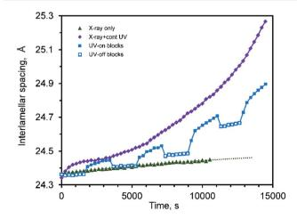
Fig. 8 Interlamellar spacing of CTA-W<sub>12</sub> as a function of time irradiated with X-rays only, X-rays plus UV, and intermittent UV.
