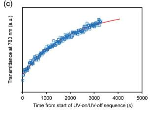
Fig. 3 Photochromic behavior of CTA-W<sub>12</sub>. (a) Plot of diffuse reflectance at 783 nm vs. photochromic cycles. (b) Diffuse reflectance at 783 nm vs. time for the 1<sup>st</sup> coloring cycle of a bulk powder sample showing fit of eqn (1). (c) Transmittance at 783 nm vs. time for 1st bleaching cycle of a thin coating of CTA W<sub>12</sub> on a glass slide, showing fit of eqn (1) (the vertical scales are in arbitrary units due to the nonstandard set-up of the multi-cycle experiments).
