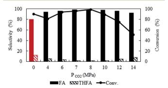
Fig. 2 Effect of CO<sub>2</sub> pressure on the conversion and selectivity of furfural hydrogenation using Pt/Al<sub>2</sub>O<sub>3</sub>. Reaction conditions: catalyst: substrate = 1:40, temperature = 80 °C,  $P_{\rm H_2} = 1$  MPa, reaction time = 4 h.
