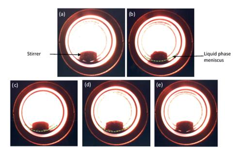
Fig. 1 Images of various phases of furfural (liquid) and  $CO_2/H_2$  (gas) observed during the reaction depending on  $CO_2$  pressure at 80 °C and hydrogen pressure of 1 MPa. (a) Empty cell, (b) furfural (c) 8 MPa, (d) 10 MPa and (e) 14 MPa.
