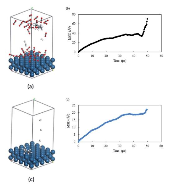
Fig. 10 Images of last frame of MD: (a) THFA in compressed  $CO_2$  and (c) THFA in solvent-less condition. Catalyst surface = teal, hydrogen = white, carbon = grey and oxygen = red. MSD plot of THFA in (b) compressed  $CO_2$  and (d) solvent-less condition.
