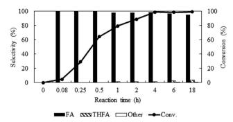
Fig. 6 Time profile of furfural hydrogenation in compressed  $CO_2$ . Reaction conditions: catalyst:substrate = 1:40, temperature =  $80 \, ^{\circ}$ C,  $P_{CO_2} = 8$  MPa,  $P_{H_2} = 1$  MPa.
