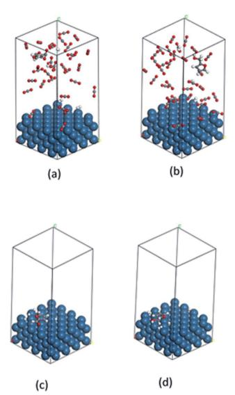
Fig. 9 Calculated images of adsorption: (a) furfural, (b) furfuryl alcohol in compressed  $CO_2$  and (c) furfural, (d) furfuryl alcohol in solvent-less condition on the catalyst surface. Color code: catalyst surface = teal, hydrogen = white, carbon = grey and oxygen = red.
