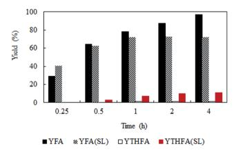
Fig. 8 Time dependent yield of furfuryl alcohol and THFA. Reaction conditions: catalyst: substrate = 1:40, temperature = 80 °C,  $P_{\rm H_2}$  = 1 MPa. YFA = yield of furfuryl alcohol, YTHFA = yield of THFA in compressed CO<sub>2</sub>; YFA (SL) = yield of furfuryl alcohol and YTHFA (SL) = yield of THFA in solvent-less condition.
