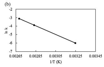
Fig. 4 (a) Temperature dependent activity and selectivity and (b) Arrhenius plot: reaction conditions: catalyst: substrate = 1:40,  $P_{\text{CO}_2} = 8$  MPa,  $P_{\text{H}_3} = 1$  MPa, reaction time = 4 h.
