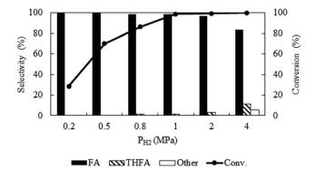
Fig. 3 Optimization of hydrogen pressure of furfural hydrogenation in compressed CO<sub>2</sub>. Reaction conditions: catalyst: substrate = 1:40, temperature = 80 °C,  $P_{\text{CO}_2} = 8$  MPa, reaction time = 4 h.
