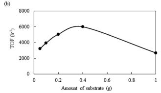
Fig. 5 Effect of the variation of substrate amount on the conversion and selectivity: reaction conditions: catalyst = 0.01 g, temperature =  $80\,^{\circ}$ C,  $P_{\text{CO}_2} = 8$  MPa,  $P_{\text{H}_2} = 1$  MPa, reaction time = 4 h.
