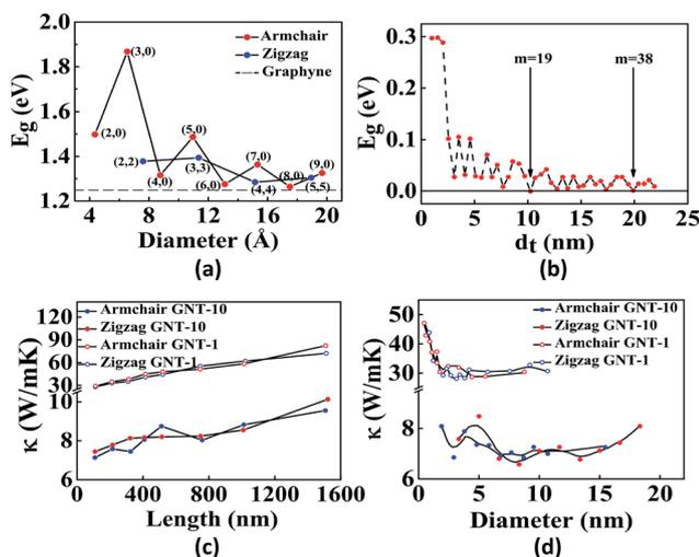
**Fig. 2** Representative properties of GNTs: effect of tube diameter on the band gap of (a)  $\gamma$ -GNTs and (b) zigzag  $\beta$ -GNTs. Dependence of the thermal conductivity on (c) tube length and (d) tube diameter of various GNTs. Part a is reproduced from ref. 51 with permission from the American Chemical Society. Part (b) is reproduced from ref. 59 and parts (c) and (d) are reproduced from ref. 55 with permissions from the American Physical Society.
