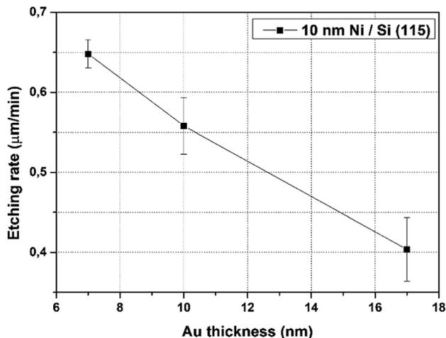
Fig. 5 The dependence of etching rate of Si (115) substrates on Au layer thickness in MaCE process (10 nm Ni), concentration of HF – 10%, H<sub>2</sub>O<sub>2</sub> – 2.5%, etching time 5 min.
