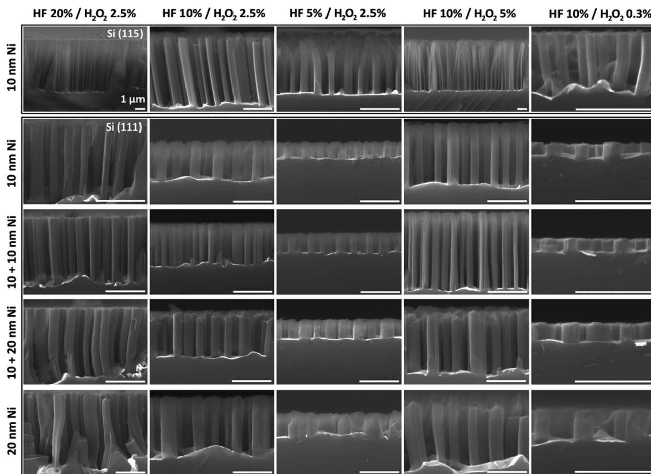
Fig. 3 SEM images of the effect of the metal-assisted wet chemical etching of Si (111) and Si (115) substrates in solutions with different HF and  $\text{H}_2\text{O}_2$  concentrations. Thickness of Au layer was 10 nm. Scale bar – 1  $\mu\text{m}$ .
