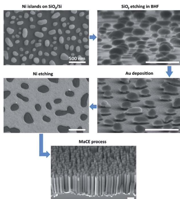
Fig. 1 Technological process flowchart of Si substrates nanostructuring, following stages: solid-state dewetting of Ni layer, etching of  $\text{SiO}_2$  layer in BHF solution, deposition of Au layer, etching of Ni islands in HF solution, MaCE process of Si substrate. Scale bar – 500 nm.
