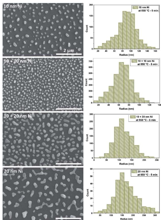
Fig. 2 SEM images of the 10 nm, 10 nm + 10 nm, 10 nm + 20 nm and 20 nm Ni layers on  $\text{SiO}_2/\text{Si}$  substrates annealed at 850 °C temperature and the histograms of Ni islands radius. Scale bar – 2  $\mu\text{m}$ .
