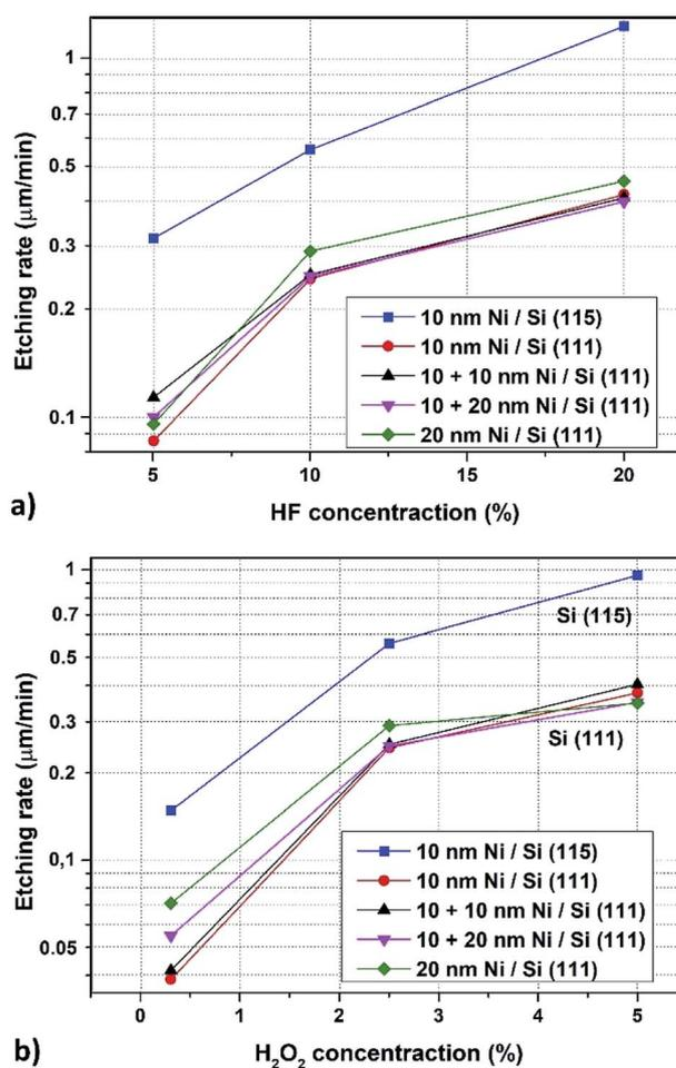
**Fig. 4** The dependence of etching rate of Si (111) and Si (115) substrates on HF concentration in the MaCE process, concentration of H<sub>2</sub>O<sub>2</sub> – 2.5% (a); the dependence of etching rate of Si (111) and Si (115) substrates on H<sub>2</sub>O<sub>2</sub> concentration in MaCE process, concentration of HF – 10% (b).
