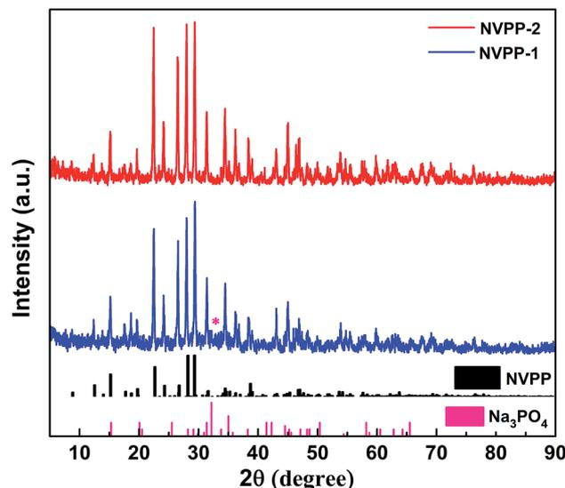
Fig. 1 Powder XRD patterns of NVPP.
