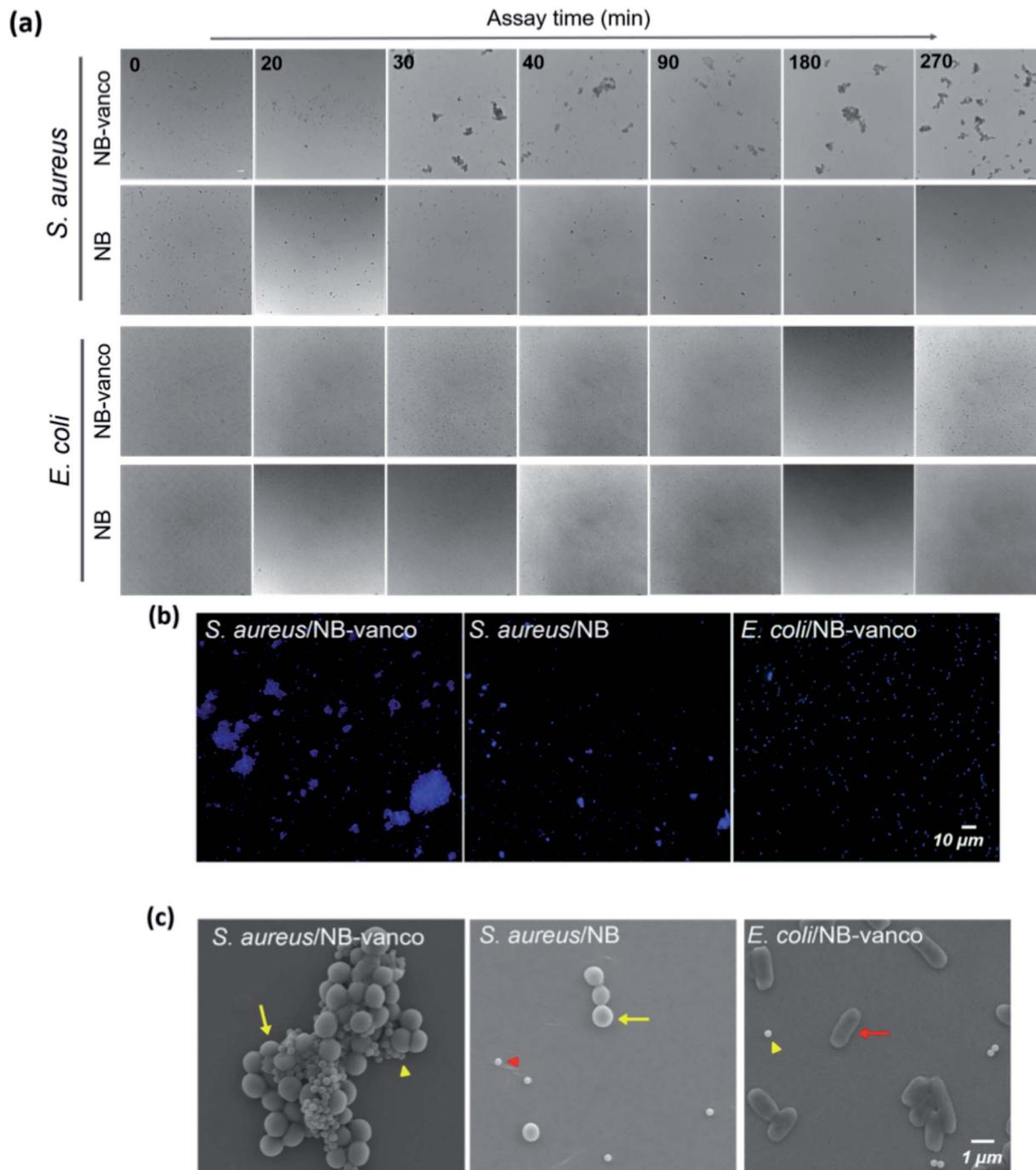
Fig. 4 Characterization of the nano-aggregates by microscopy. (a) Bright field images of the nano-aggregates according to various assay time (scale bar, 25 μm). (b) Fluorescence microscopy (blue: DAPI) and (c) scanning electron microscopy of the nano-aggregates (arrows: yellow – *S. aureus*, red – *E. coli*; arrowheads: yellow – NB-vanco, red – NB).
