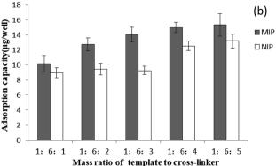
Fig. 2 Adsorption capacities of the MIP and NIP films synthesized at different mass ratios of template to functional monomer (a); and different mass ratios of template to cross-linker (b).
