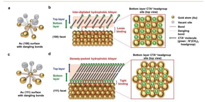
Fig. 5 Schematic of the CTA<sup>+</sup> bilayer structure according to the facet of Au NPs. (a) One Au (100) surface atom with dangling bonds. (b) Interdigitated hydrophobic CTA<sup>+</sup> bilayer structure on the (100) facet. (c) One Au (111) surface atom with dangling bonds. (d) Densely packed hydrophobic CTA<sup>+</sup> bilayer structure on the (111) facet. The CTA<sup>+</sup> molecule headgroup adhesion site is denoted in the schematic as green balls.
