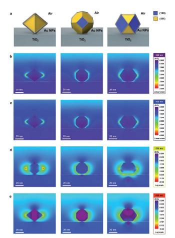
Fig. 1 FDTD simulation results ( $|E/E_0|$ ) of the three kinds of Au nanoparticles (octahedral, truncated octahedral and cuboctahedral) at various incident wavelengths. (100) and (111) facets are denoted as yellow and blue, respectively. (a) Schematic configurations of Au nanoparticles. (b) Field enhancement at 350 nm photons. (c) Field enhancement at 450 nm photons. (d) Field enhancement at 550 nm photons. (e) Field enhancement at 650 nm photons.
