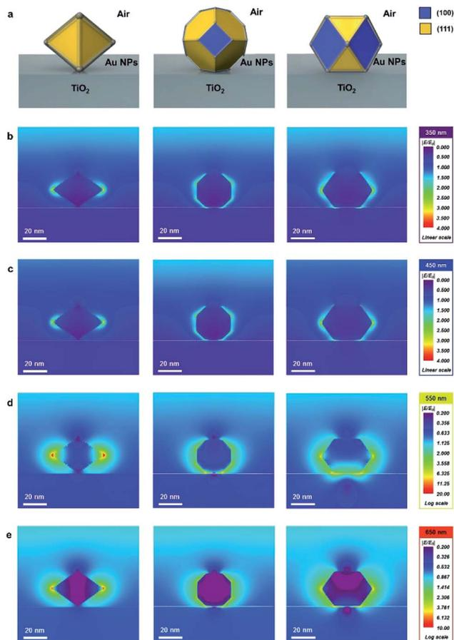
Fig. 1 FDTD simulation results ( $|E/E_0|$ ) of the three kinds of Au nanoparticles (octahedral, truncated octahedral and cuboctahedral) at various incident wavelengths. (100) and (111) facets are denoted as yellow and blue, respectively. (a) Schematic configurations of Au nanoparticles. (b) Field enhancement at 350 nm photons. (c) Field enhancement at 450 nm photons. (d) Field enhancement at 550 nm photons. (e) Field enhancement at 650 nm photons.
