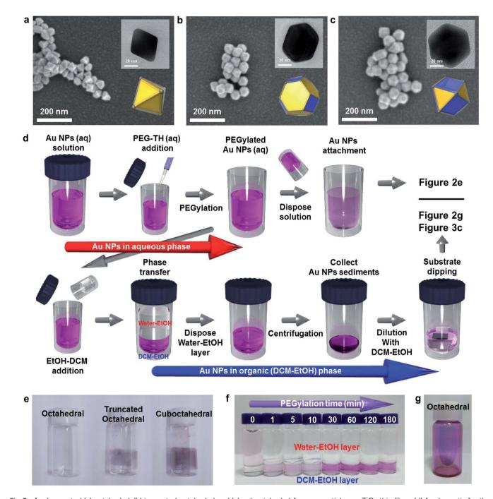
Fig. 2 Agglomerated (a) octahedral, (b) truncated octahedral and (c) cuboctahedral Au nanoparticles on TiO<sub>2</sub> thin films. (d) A schematic for the process of anchoring Au nanoparticles for the semiconductor nanostructure attachment using PEGylation in agueous phase and phase transfer to organic medium. (e) A visualization of the Au NP attachment using vials. (f) Phase transfer to organic medium according to the PEGylation time. (g) Image of octahedral Au nanoparticles attached to a vial.
