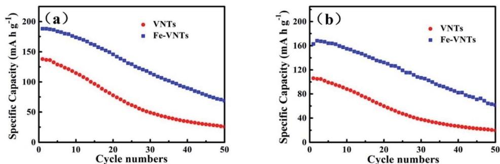
Fig. 10 Cycling performance of VNT and Fe-VNT at (a) 50 mA g<sup>-1</sup> (b) 80 mA g<sup>-1</sup>.
