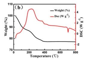
Fig. 5 The thermos-gravimetric analyses (TGA) of (a) VNTs (b) Fe-VNTs.
