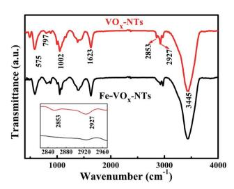
Fig. 6 FTIR spectra of VNTs and Fe-VNTs. Inset is the zoom area of two peaks located at 2835 and 2917 cm<sup>-1</sup>.
