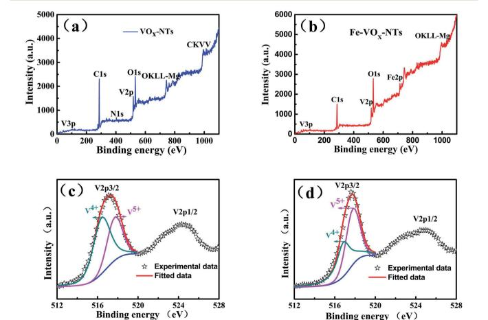
Fig. 7 XPS general spectrum (a) and V2p region (c) of the VNTs, and XPS general spectrum (b) and V2p region (d) of the Fe-VNTs.
