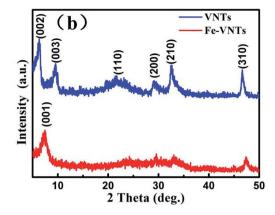
Fig. 3 Small-angle (a) and wide-angle (b) XRD patterns of VNTs and Fe-VNTs.
