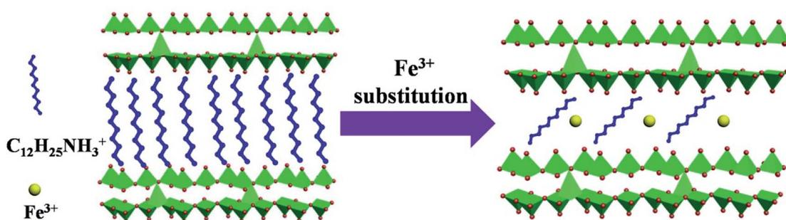
Fig. 4 Schematic illustration of the ferric ion substitution.
