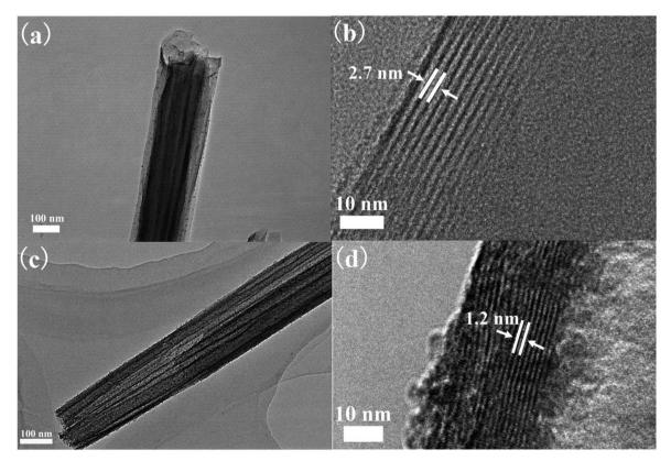
Fig. 2 TEM images of (a and b) VNTs (c and d) Fe-VNTs at different magnifications.
