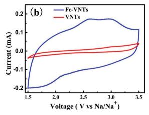
Fig. 9 (a) Galvanostatic charge—discharge profiles of first cycle of VNTs and Fe-VNTs between 1.5-3.5 V at 50 mA  $\rm g^{-1}$ . (b) Cyclic voltammograms of VNTs and Fe-VNTs at scan rate of 0.5 mV  $\rm s^{-1}$ .
