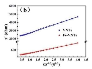
Fig. 11 (a) Nyquist plots of VNTs and Fe-VNTs. (b) The fitted lines and real part of the impedance versus  $\omega^{-1/2}$  for VNTs and Fe-VNTs.
