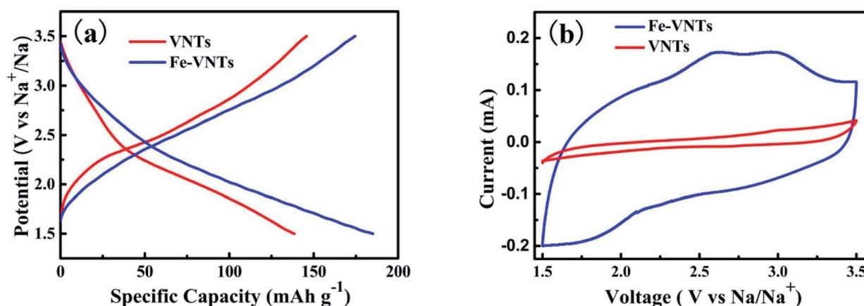
Fig. 9 (a) Galvanostatic charge–discharge profiles of first cycle of VNTs and Fe-VNTs between 1.5–3.5 V at  $50 \text{ mA g}^{-1}$ . (b) Cyclic voltammograms of VNTs and Fe-VNTs at scan rate of  $0.5 \text{ mV s}^{-1}$ .
