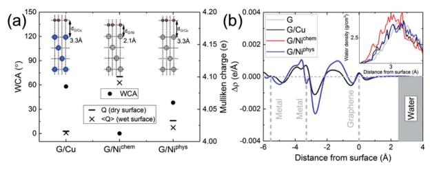
Fig. 3 Calculated for graphene on Cu (111), (chemisorbed) Ni (111) and (physisorbed) Ni (111) metal substrates: (a) •: WCA; — and ×: Mulliken charge before (dry) and after (wet) water wetting; (b) planar-averaged electron density difference and water density profile (inset).
