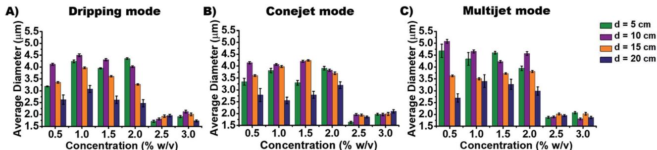
Fig. 4 The measured average particle diameters for different concentrations in electro-spray modes. (A)–(C) Average diameter ( $\mu\text{m}$ ) vs. concentration (% w/v) with increasing concentration of Na-Alg in water : ethanol = 8 : 2 solution for dripping mode (A), conejet mode (B) and multijet mode (C). All plotted error bars are representing the standard error.
