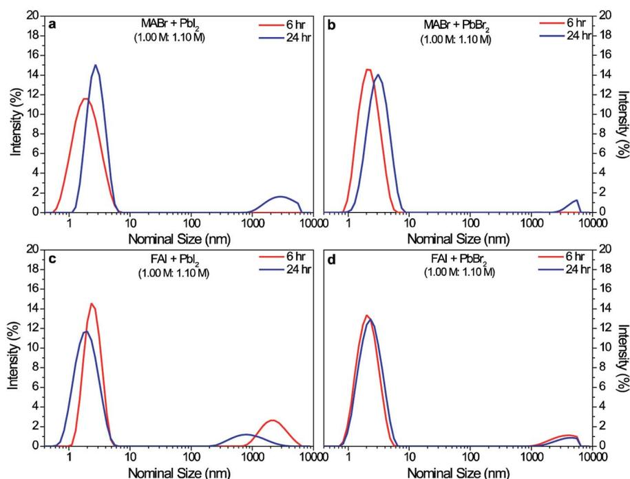
Fig. 4 DLS data of precursor solutions containing (a) MABr + PbI<sub>2</sub>, (b) MABr + PbBr<sub>2</sub>, (c) FAI + PbI<sub>2</sub>, (d) FAI + PbBr<sub>2</sub> with respect to its precursor solution aging time.
