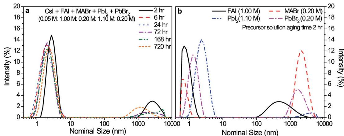
Fig. 3 DLS data of (a) triple-cation lead halide perovskite (FAI + MABr + PbI<sub>2</sub> + PbBr<sub>2</sub> + CsI) and (b) single precursor components at the solution aging time of 2 h.
