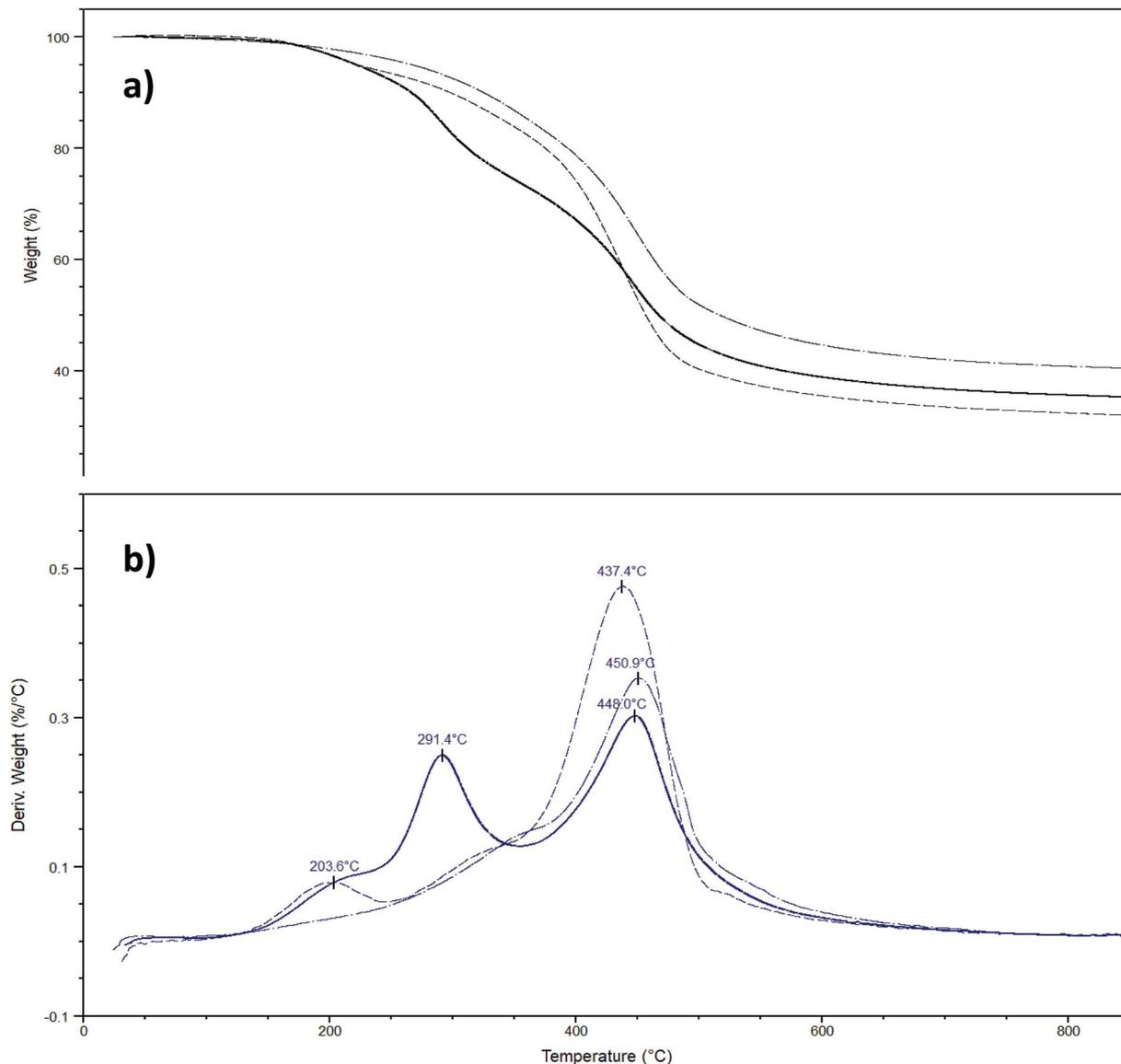
Fig. 5 a) Temperature-ramped TGA thermographs of CPS-SEC (dash dot line), IL functionalized sporopollenin **5b** (solid line) and IL functionalized sporopollenin **6b** (short dash line) with a heating rate of  $10\text{ }^{\circ}\text{C min}^{-1}$ . (b) Temperature-ramped TGA thermographs of CPS-SEC (dash dot line), IL functionalized sporopollenin **5b** (solid line) and IL functionalized sporopollenin **6b** (short dash line).
