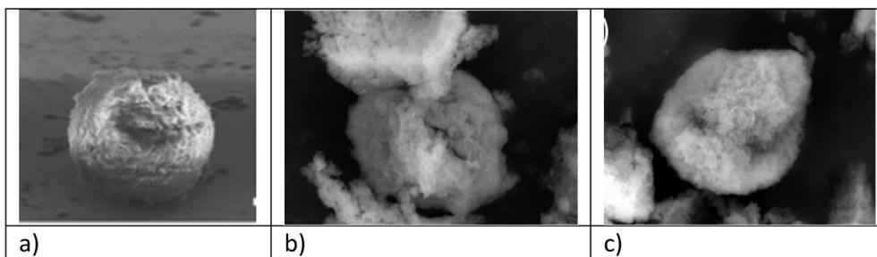
Fig. 3 SEM images of (a) sporopollenin extracted with the IL  $[\text{HSO}_3\text{C}_4\text{mim}][\text{HSO}_4]$ , (b) 3-chloropropyl-functionalized sporopollenin CPS-SEC and (c) IL-functionalized sporopollenin **5b**.
