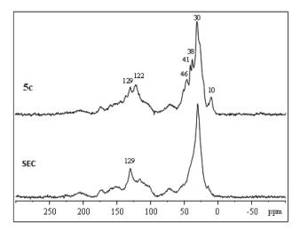
Fig. 4 <sup>13</sup>C CP-MAS NMR spectrum of sporopollenin (SEC) and IL-functionalized sporopollenin **5a**.
