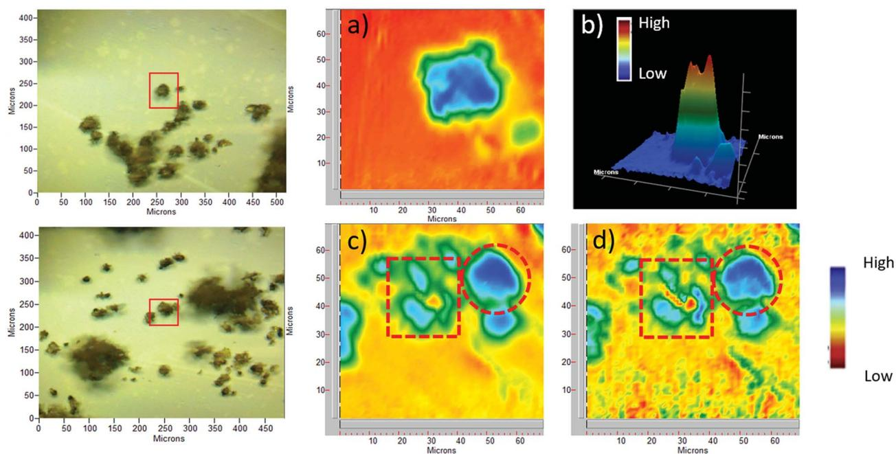
Fig. 2 Optical and FPA images: (a) 2D image (blue is high) of 3-chloropropyl-functionalized sporopollenin CPS-SEC, selected wavenumber  $1035\text{ cm}^{-1}$ ; (b) 3D image (red is high) of CPS-SEC; (c) 2D image of IL-functionalized sporopollenin **5b** at  $1035\text{ cm}^{-1}$ ; (d) 2D image of **5b** at  $1563\text{ cm}^{-1}$ . Red circles indicate intact pollen grains, whereas red squares show pollen fragments.
