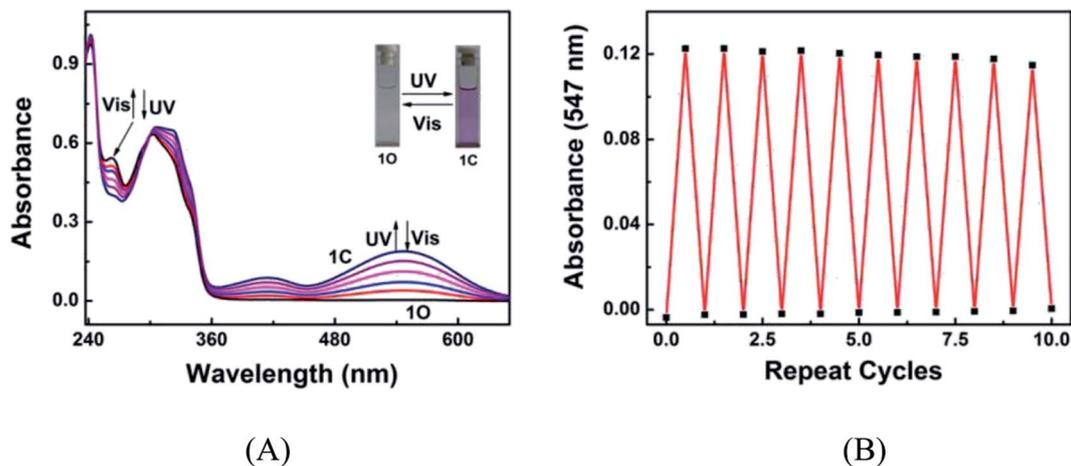
Fig. 1 (A) Changes in the absorption spectrum of 1O in acetonitrile ( $2.0 \times 10^{-5} \text{ mol L}^{-1}$ ) upon alternating irradiation with UV and visible light; (B) fatigue resistance of 1O in acetonitrile under the alternating irradiation at room temperature.
