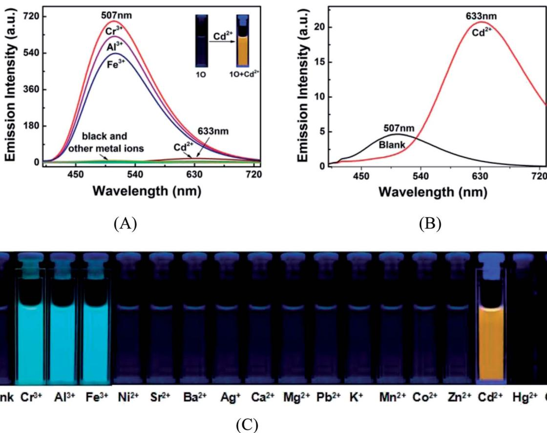
Fig. 3 Fluorescence changes of **10** (2.0 × 10<sup>-5</sup> mol L<sup>-1</sup>) in acetonitrile in response to various metal ions (2.4 equiv.). (A) Fluorescence emission spectra of **10** in the presence of various metal ions; (B) fluorescence emission spectra of **10** in the presence of Cd<sup>2+</sup>; (C) image demonstrating the solution color of **10** in the presence of different metal ions.
