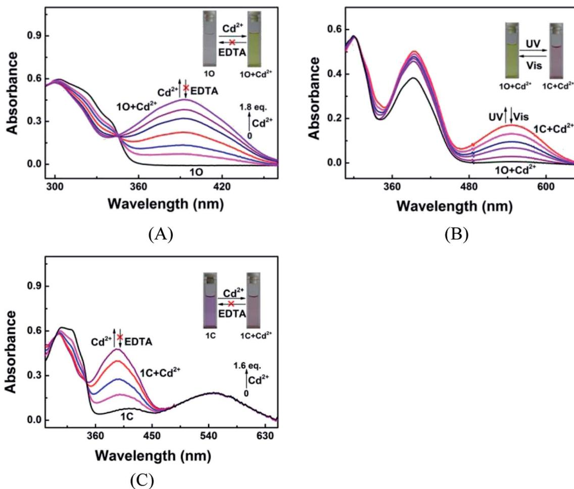
Fig. 2 Changes in the absorption spectrum and color of 1O in acetonitrile ( $2.0 \times 10^{-5} \text{ mol L}^{-1}$ ) in response to  $\text{Cd}^{2+}$ /EDTA and light stimuli. (A) Spectral changes of 1O induced by  $\text{Cd}^{2+}$ /EDTA; (B) spectral changes of 1O +  $\text{Cd}^{2+}$  induced by UV/vis light; (C) spectral changes of 1C induced by  $\text{Cd}^{2+}$ /EDTA.
