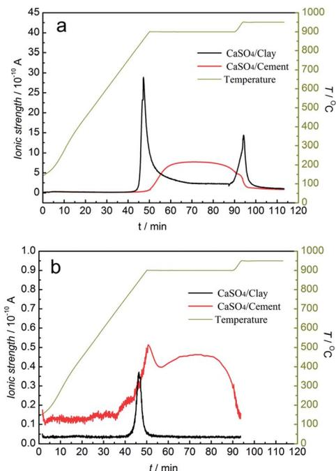
Fig. 8 Mass spectrometric analysis of sulphurous gas products from TGA with steam as the gasifying agent. (a) SO<sub>2</sub>; (b) H<sub>2</sub>S.
