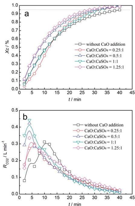
Fig. 9 Variation of carbon conversion efficiency (a) and CO<sub>2</sub> generation rate (b) with time for the CaSO<sub>4</sub>/clay composite oxygen carrier with different CaO additions.
