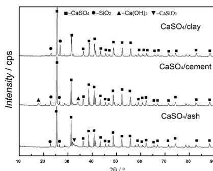
Fig. 3 XRD patterns of fresh composite oxygen carrier.
