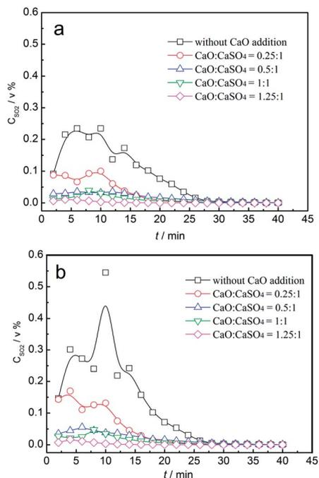
Fig. 10 Variation of gas concentrations of SO<sub>2</sub> with time for the CaSO<sub>4</sub>/clay composite oxygen carrier with different CaO additions; (a) reduction stage, (b) oxidation stage.
