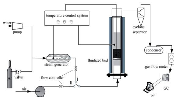
Fig. 1 Schematic diagram of the experimental fluidised-bed setup.
