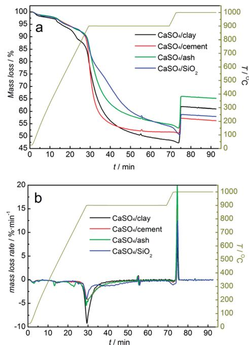
Fig. 6 TG (a) and DTG (b) curves of composite oxygen carriers undergoing one redox cycle with coal using steam as the gasifying agent and air, alternately.
