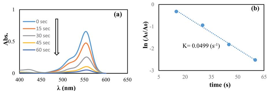
Fig. 12 The reduction of RhB in aqueous solution recorded every 15 s using the Pd NPs/RGO nanocomposite (1 mg) as a catalyst (a)  $\ln(A_t/A_0)$  versus reaction time for the reduction of RhB (b).
