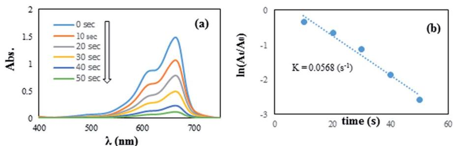
Fig. 11 The reduction of MB in aqueous solution recorded every 10 s using the Pd NPs/RGO nanocomposite (1 mg) as a catalyst (a)  $\ln(A_t/A_0)$  versus reaction time for the reduction of MB (b).
