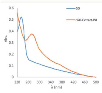
Fig. 2 UV-vis spectra of the GO and RGO.
