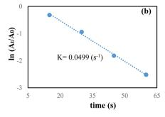
Fig. 12 The reduction of RhB in aqueous solution recorded every 15 s using the Pd NPs/RGO nanocomposite (1 mg) as a catalyst (a)  $\ln(A_t/A_0)$  versus reaction time for the reduction of RhB (b).
