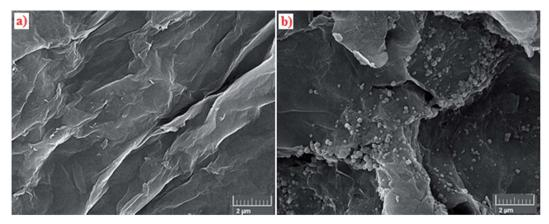
Fig. 3 (a) FE-SEM images of GO, and (b) Pd NPs/RGO.
