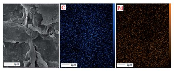
Fig. 5 FE-SEM image of Pd NPs/RGO and elemental maps of C, and Pd atoms.
