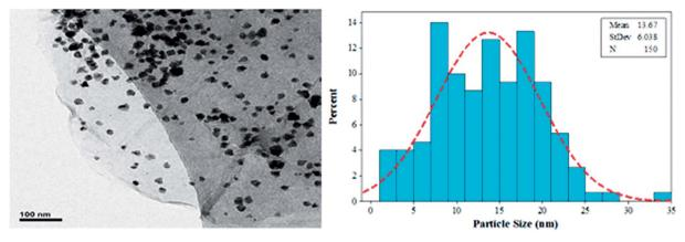
Fig. 7 TEM image of Pd NPs/RGO with Pd NP size distributions
