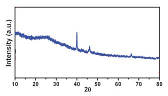
Fig. 8 XRD pattern of Pd NPs/RGO.
