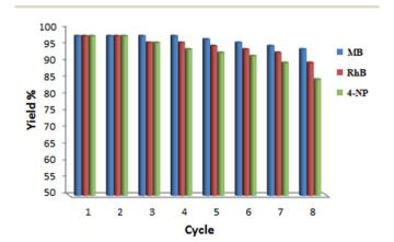
Fig. 13 Reusability of the Pd NPs/RGO nanocatalyst for the reduction of MB, RhB and 4-NP in the presence of NaBH $_4$ .
