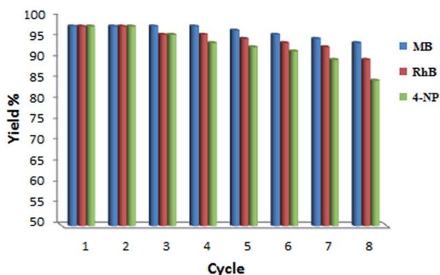
Fig. 13 Reusability of the Pd NPs/RGO nanocatalyst for the reduction of MB, RhB and 4-NP in the presence of NaBH<sub>4</sub>.
