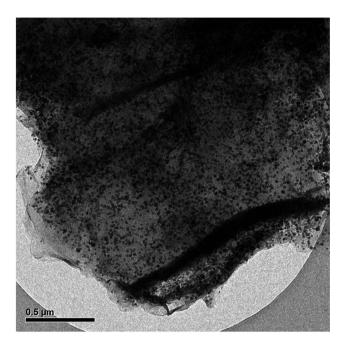
Fig. 6 TEM image of Pd NPs/RGO
