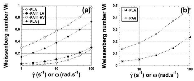
Fig. 8 The Weissenberg number *versus* angular frequency at 200 °C (a) for neat PLA, PA11, PLA-j samples; at 230 °C (b) for neat PLA and PA6 samples.
