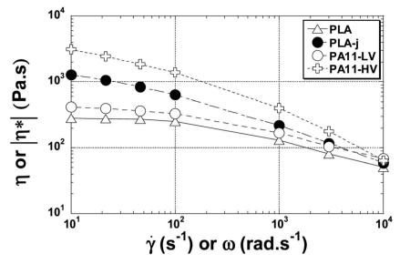
Fig. 10 The viscosity shear rate dependence at 200 °C for neat, modified PLA and PA11.
