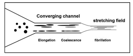
Fig. 14 Schematic illustration of morphological evolution of in situ nanofibrillar PLA-j-PA11 blends.
