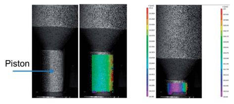
Fig. 4 Schematic illustration of the digital image correlation during microinjection process.
