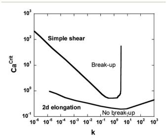
Fig. 1 The Grace curve gives the relation between the critical capillary number  $Ca_{(crit)}$  and the viscosity ratio k for the breakup of an initially spherical droplet in quasi-steady homogeneous flow (in simple shear and plane hyperbolic flow).4
