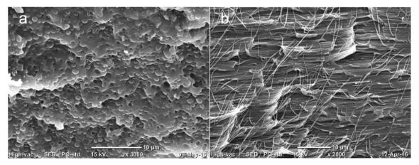
Fig. 11 SEM observation of longitudinal fracture surfaces of extrudates for (a) PLA/PA11-LV, (b) PLA-i/PA11-LV.
