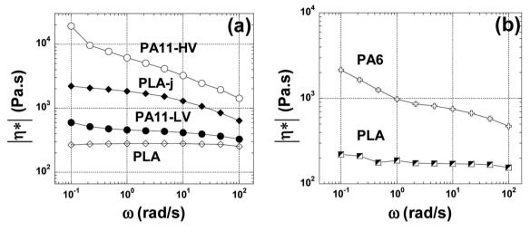
Fig. 6 The complex viscosity angular frequency dependence at 200  $^{\circ}$ C for neat, modified PLA and PA11 samples (a) and for neat PLA, PA6 at 230  $^{\circ}$ C (b).
