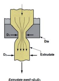
Fig. 5 Schematization of the extrudate swell measurement at the die exit.
