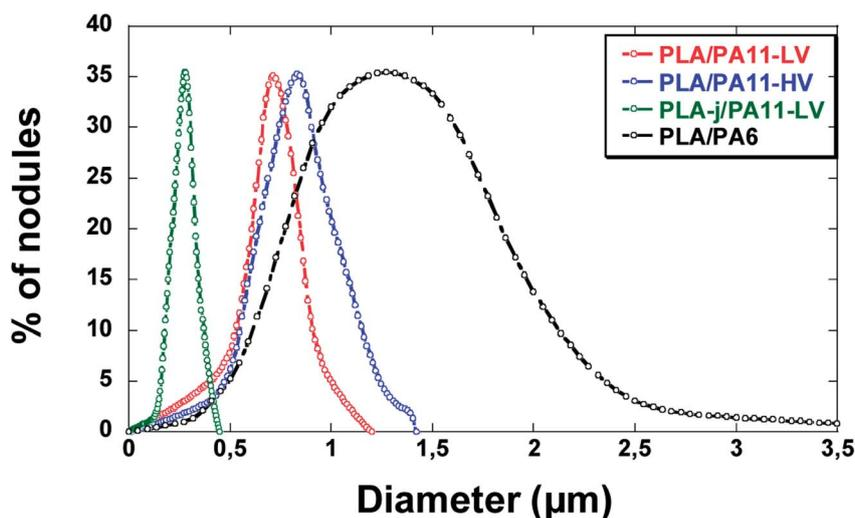
Fig. 13 Particle size distribution of PLA/PA blends.
