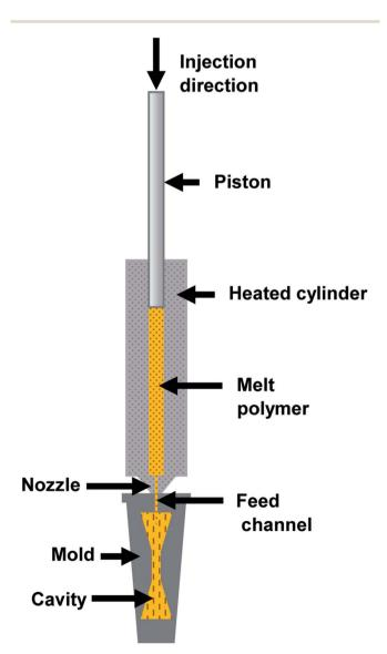
Fig. 3 Schematic illustration of the piston micro-injection process.
