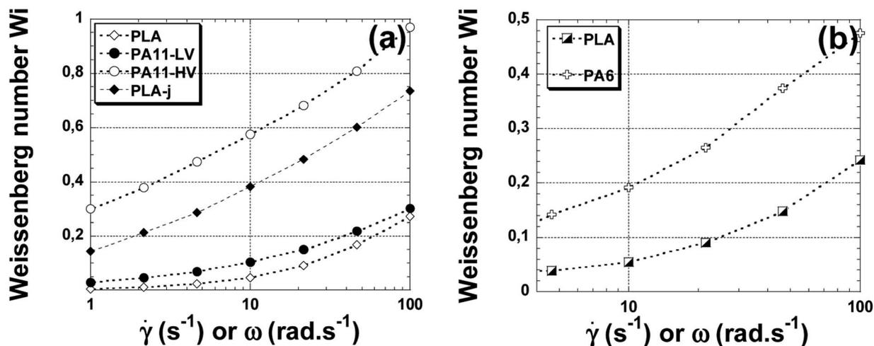
Fig. 8 The Weissenberg number versus angular frequency at 200 °C (a) for neat PLA, PA11, PLA-j samples; at 230 °C (b) for neat PLA and PA6 samples.
