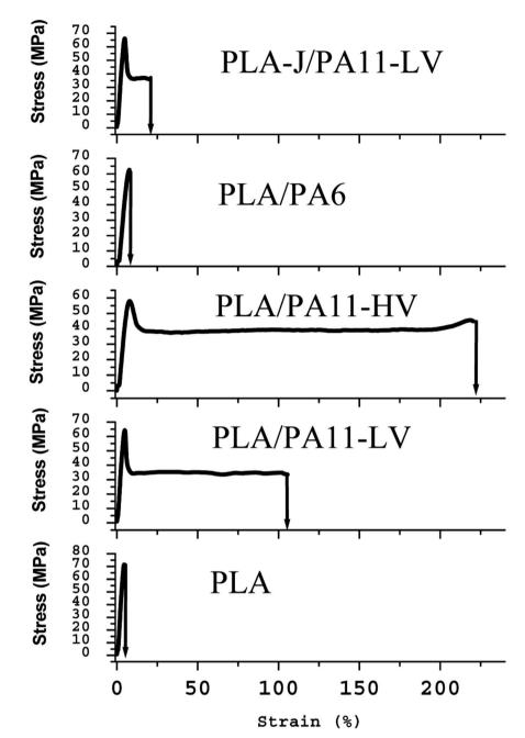
Fig. 19 Tensile stress versus tensile strain of neat PLA and various polymer blends
