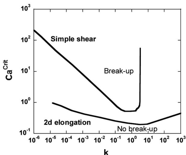
Fig. 1 The Grace curve gives the relation between the critical capillary number  $Ca_{(crit)}$  and the viscosity ratio  $k$  for the breakup of an initially spherical droplet in quasi-steady homogeneous flow (in simple shear and plane hyperbolic flow).<sup>4</sup>
