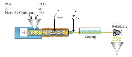
Fig. 2 Manufacturing process of polymer blends extrudates.
